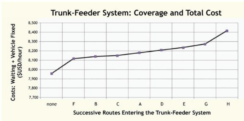
Figure 6.50. Likely total system cost curve if feeder route travel time is greater than trunk travel time. Graph *Pedro Szász*.
