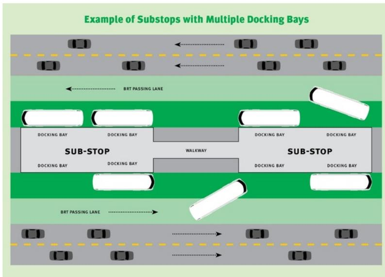
Figure 7.4. Scheme of station with two substops /ITDP
