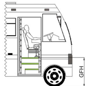
Figure 20.8. GFH 960 mm maximum Short Bus; 1,150 mm maximum Medium Bus; Front Engine High Floor; ITDP
