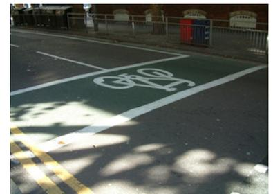
Figure 24.72. In the UK, a priority bicycle stopping area is placed ahead of the stopping line for motorized vehicles. *Lloyd Wright.*
