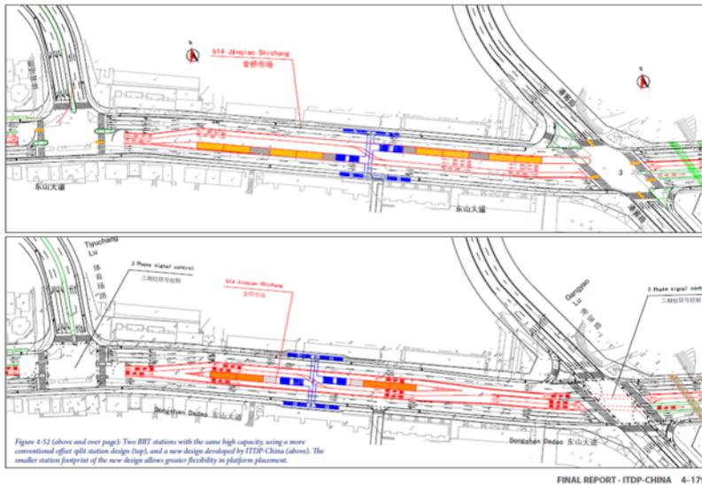
Figure 25.48. Comparison of a traditional two-sub-stop station and the new directional design applied in Lanzhou and Yichang. ITDP-China.
