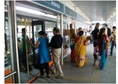
Figure 7.20. With well-designed infrastructure and adequate driver training, such as in Ahmedabad, India, BRT systems can reduce the boarding gap to under 10 centimeters Shreya Gadepalli
