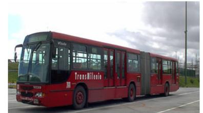
Figure 20.20. Bogotá utilizes a four-door configuration that helps to reduce boarding and alighting times. TransMilenio TM.
