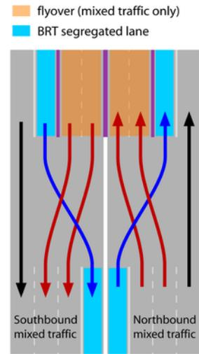
Figure 24.82. Schematic of Delhi roadway in which BRT vehicles must cross mixed traffic that is attempting to access a flyover. Image *Elebeta*.
