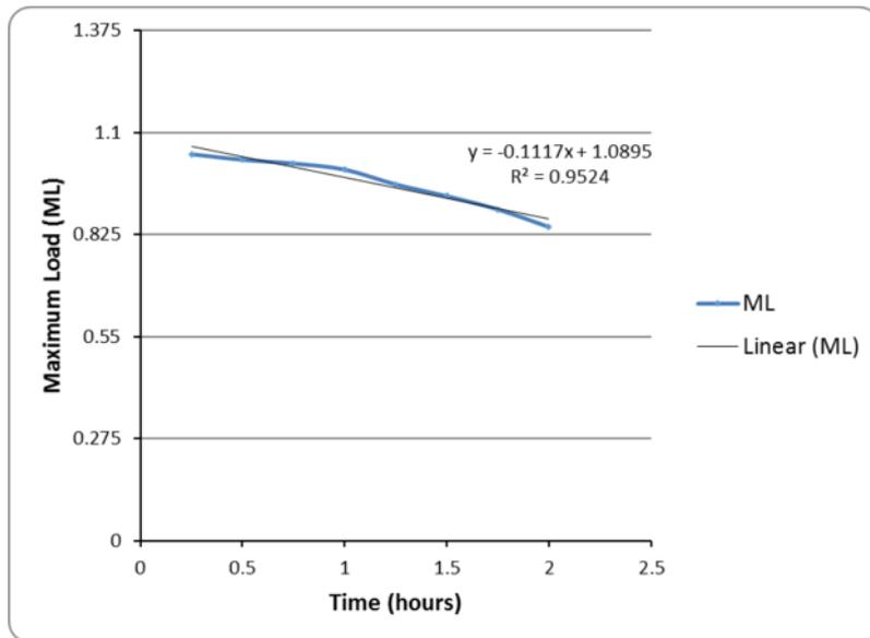
Figure 6.27. Accumulated maximum load (ML) for various cycle times as a proportion of the accumulated max load for a one-hour cycle time. The slope, as shown by the formula and the straight black line, represents the PHtoCC. Image Arthur Szász.
