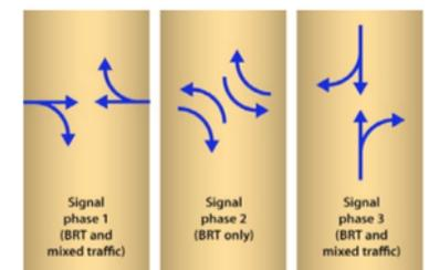
Figure 24.55. In order to permit the BRT turning movements suggested in Figure 24.54, a three-phase traffic signal would be required. ITDP.
