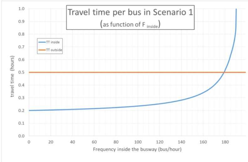
Figure 6.35. Scenario I travel time inside the BRT corridor (blue line) and outside the BRT corridor (orange line) as a function of bus frequency brought inside the corridor. *Elebeta*.
