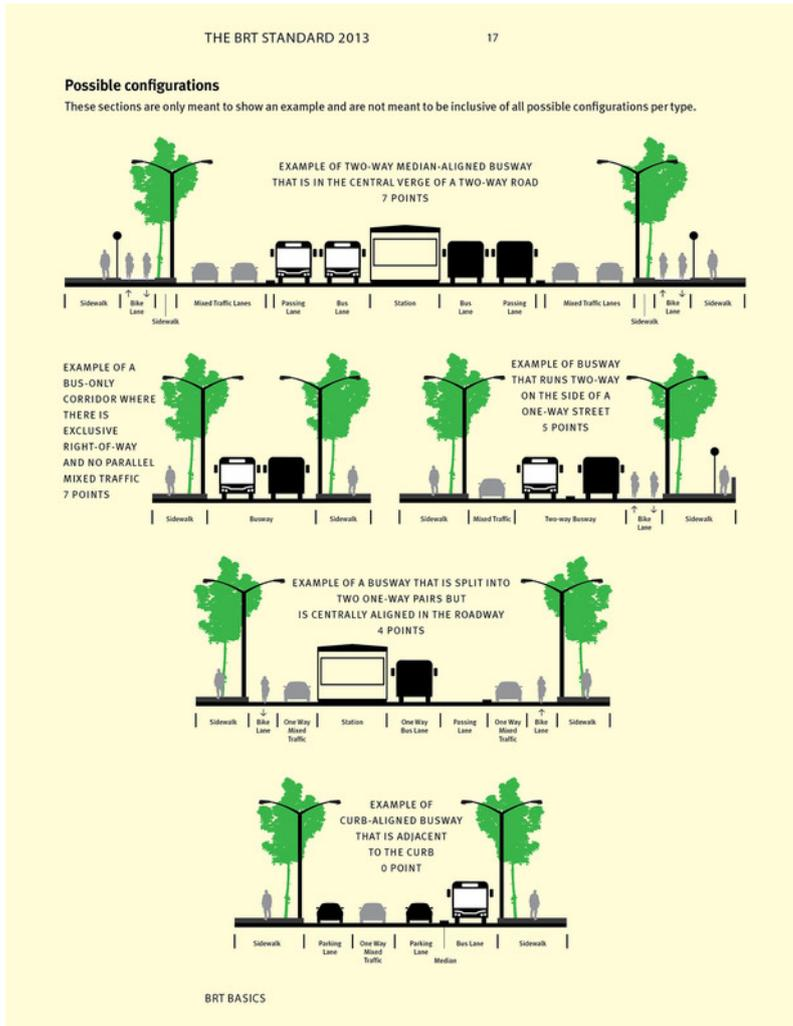
Figure 22.8. Examples of different BRT roadway configurations from The BRT Standard. *ITDP*.
