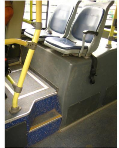
Figure 30.51. Irregular seating plans reduce internal accessibility. *Tom Rickert/AEI.*
