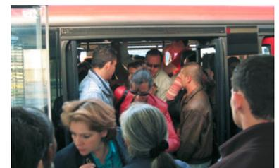
Figure 7.30. The overcrowding of vehicles results in delayed boarding and alighting due to customer congestion around the doorway (Bogotá). Image Carlosfelipe Pardo.
