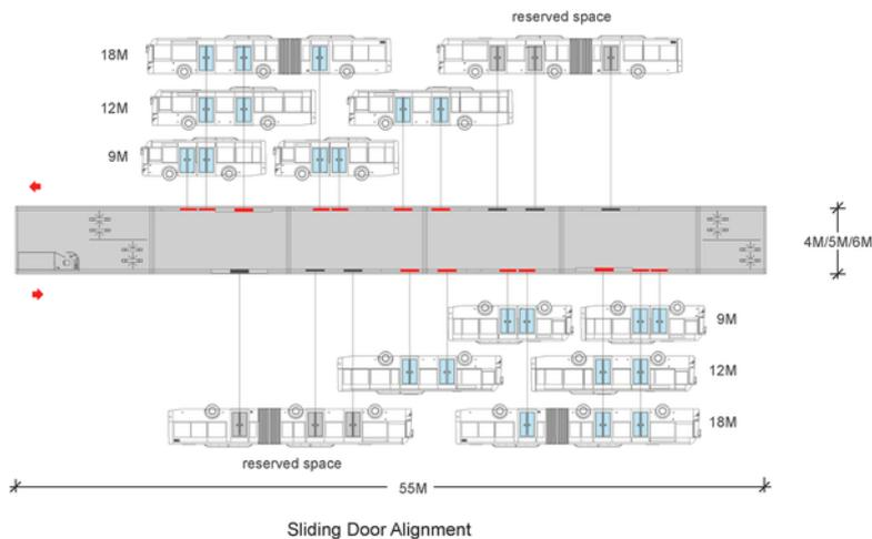
Figure 25.88. Location and alignment of sliding doors in proposed BRT stations in Vientiane. There are other types of stations; this 55-meter station is the standard one. *ITDP-China*
