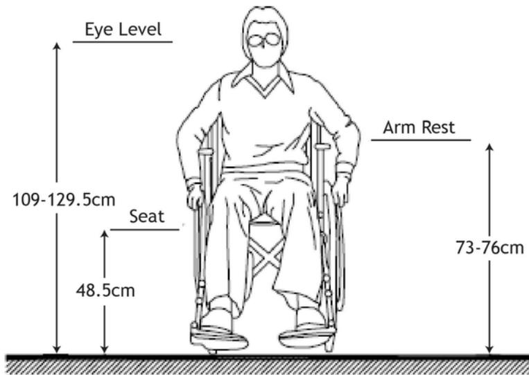
Figure 20.21. Wheelchair dimensions and the anthropometric measurements indicated in the preceding diagrams should be considered in sizing the backrest. ITDP
