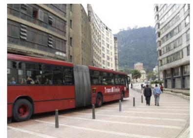
Figure 23.25. Along Bogotá's Alameda Jiménez, bollards separate the busway from the pedestrian walkway. Diego Velazquez
