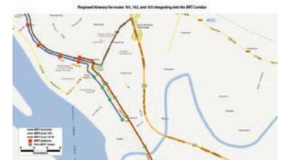
Figure 6.71. The need for transfers is also reduced when local routes are overlapping in the CBD, zoom of proposed design in Yichang CBD. ITDP.
