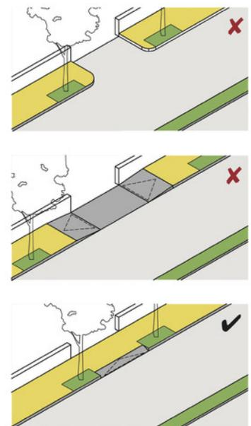
**Figure 29.17.** Where required to enable access to private properties, curb cuts should be provided in the landscaping strip, but not in the area of pedestrian through-movement. Ending the footpath with abrupt curbs, or lowering the entire footpath to the level of the roadway is unacceptable as property entrances may become waterlogged. *ITDP’s Better Streets, Better Cities (2011)*
