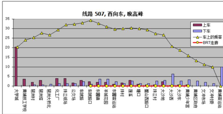
Figure 4.14. This is the display of a survey result taken in 2006 before the Guangzhou BRT was built. It shows the boarding and alighting along bus route 507. The stops with yellow dots connected with a red line are stops along the planned Zhongshan Road BRT system, with the line at the top showing bus occupancy. ITDP.
