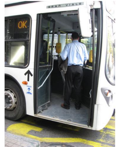
Figure 20.10. Low-floor vehicles without platform-level entry and pre-board fare verification can result in longer dwell times and not actually provide access to the physically disabled, as shown in this image from Santiago, Chile Lloyd Wright
