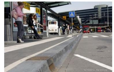
Figure 25.93. Smooth, hard, bevelled curb in Amsterdam to reduce tire wear. *Karl Fjellstrom*
