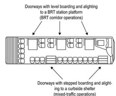
Figure 6.9. Two-sided doorway configuration for a direct-service system where the bus operates both in the BRT corridor and outside the corridor in mixed traffic. ITDP.
