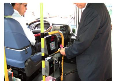
Figure 7.27. However, in Seoul, the on-board nature of the fare verification means that dwell times are negatively affected. A single customer searching through personal effects for his or her smart card can create a significant delay. Lloyd Wright.
