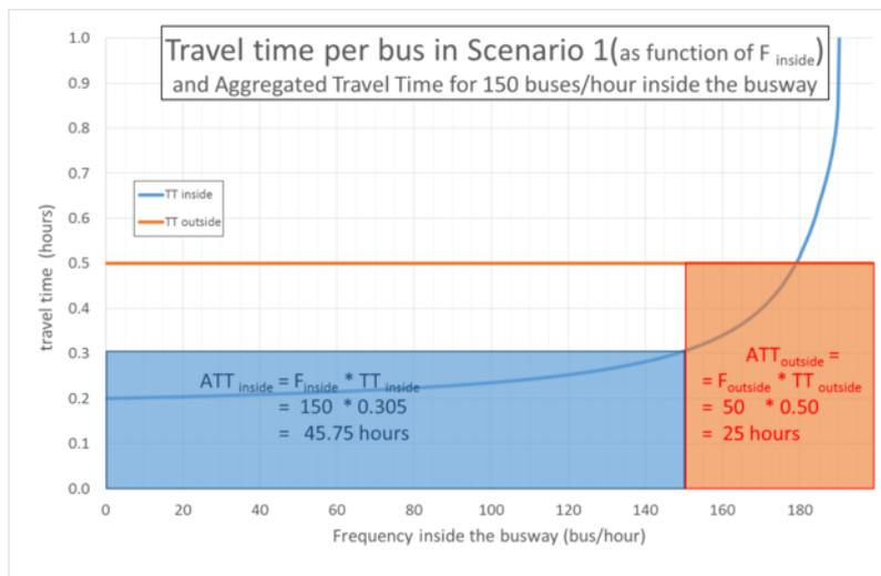
Figure 6.37. Scenario I aggregated travel times, obtained by multiplying by the fixed travel time for all buses inside the busway (0.305 hour) by the number of buses inside the busway (150, represented by the blue shading) added with the travel time outside the busway (0.50) multiplied by number of buses outside (50, represented by the orange shading), one should get  $ATT_{inside}(F_{inside} = 150) = 45.75$  hours and  $ATT_{outside}(F_{outside} = 179) = 25$  hours, respectively. *Elebeta*.
