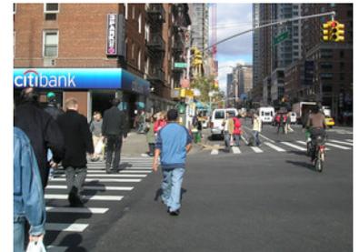
Figure 29.28. Pedestrian phase of a leading pedestrian interval in New York City. Pedestrians are permitted to begin crossing the intersection before vehicles get a green light. *Michael King*
