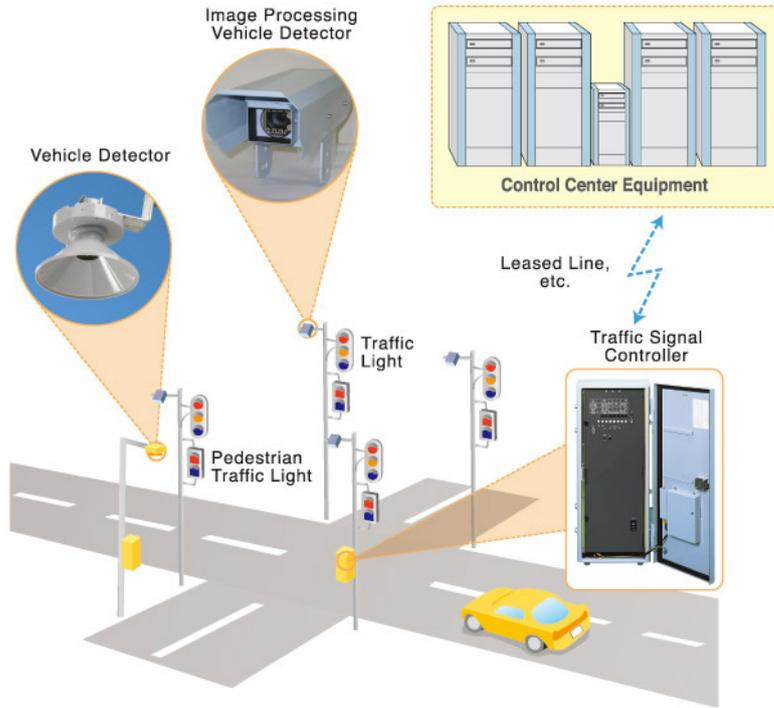
Figure 19.9. Signal control system. Sumitomo Electric.
