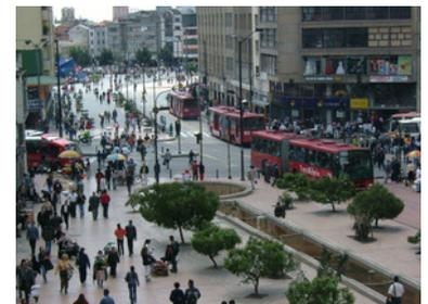
Figure 23.31. Textured and colored surface treatments help delineate pedestrian zones from roadways in Bogotá's BRT corridor. Karl Fjellstrom, Far East BRT
