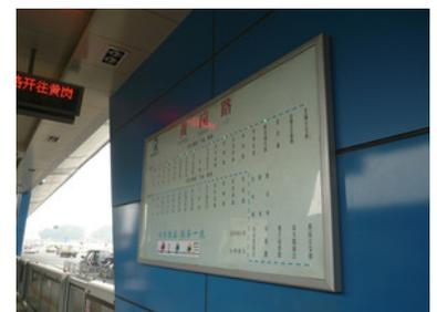
Figure 11.35. Information displays at a BRT station in the Jinan, China, system provide the real-time position of BRT buses along the corridor. Photo courtesy of ITDP.
