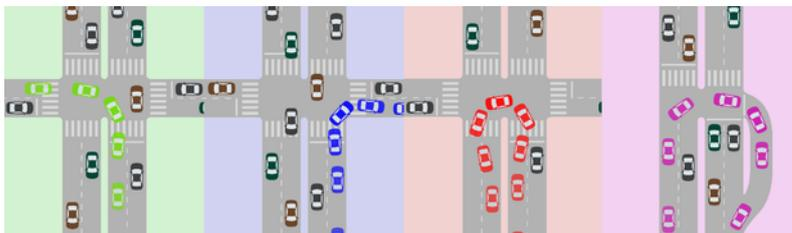
Figure 24.5. Example of a cross-traffic turn (green car), a curbside turn (blue car), a U-turn without space (red car), and a U-turn with space (pink car) for right-hand-oriented driving in China, the United States, Brazil, and most of Europe. *Elebeta*.
