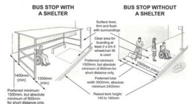
Figure 30.67. Universal design features of bus stops. Adapted by TRL from Oxley, 2002.
