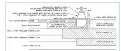
Figure 23.11. Typical pavement design for a moderately loaded concrete busway (on RHS of delineator curb), with general traffic lane (LHS of delineator curb). HHO Africa
