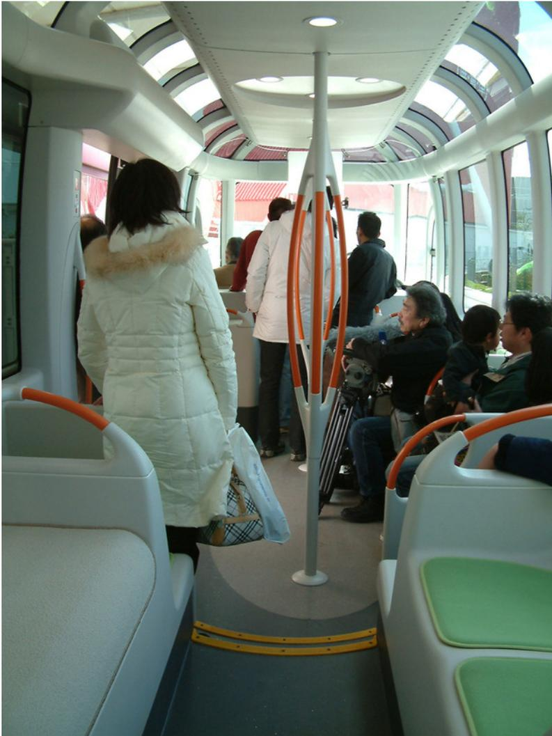
Figure 20.26. Panoramic windows, as in this bus in Aichi, Japan, can dramatically improve the customer's ability to see the outside environment. Lloyd Wright.
