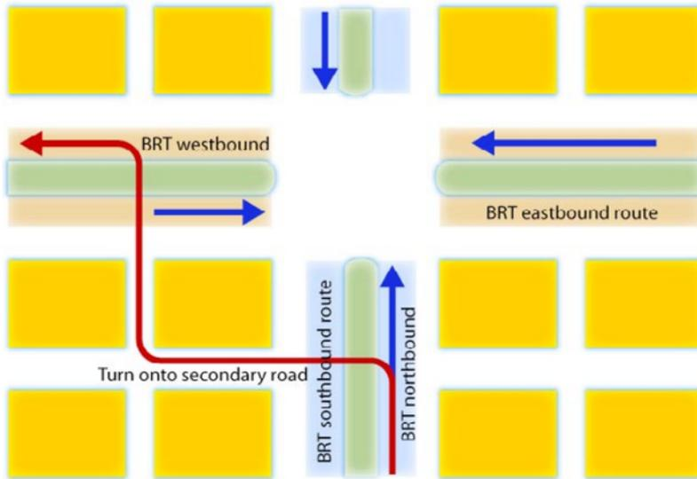
Figure 24.60. In this scenario, the BRT turning movement is made prior to the main intersection. The BRT vehicle temporarily operates on the secondary road network. ITDP.
