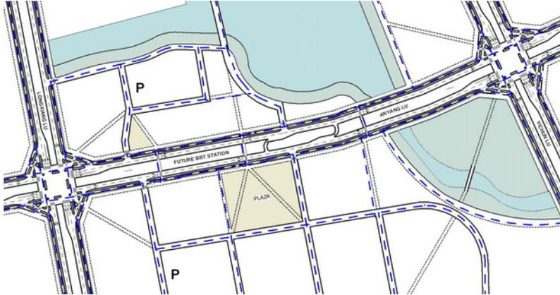
Figure 31.6. A design for a bicycle network in tandem with a BRT network in Harbin, China. Bicycle routes are denoted by dotted blue lines. Nelson\Nygaard.
