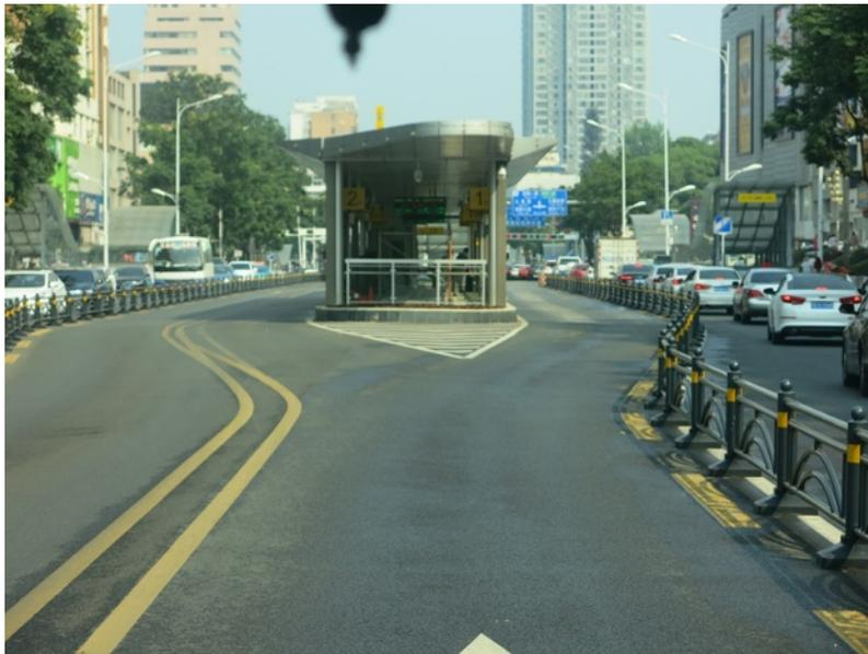
Figure 25.47. Directional BRT stations in Yichang; the buses can go on either side of the station while the opposite direction has a lane to travel past the station. *Aimee Gauthier, ITDP.*
