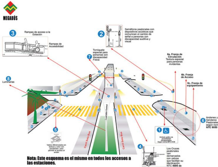
Figure 30.9. Pedestrian-access features are depicted in this diagram of approaches to a typical BRT station on Avenue Simón Bolívar in Pereira, Colombia. *Pereira Megabús.*
