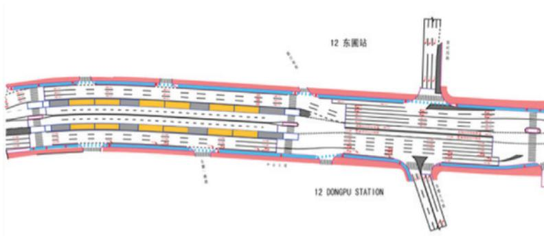
Figure 24.45. Dongpu BRT station in Guangzhou, provides at-grade station access at both ends, combined with U-turns. *ITDP with GMEDRI.*
