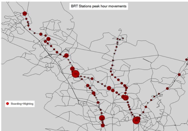
Figure 4.13. An example of peak hour existing boarding and alighting numbers mapped onto some possible BRT corridors based on APC data from Montgomery County, Maryland. *ITDP*.
