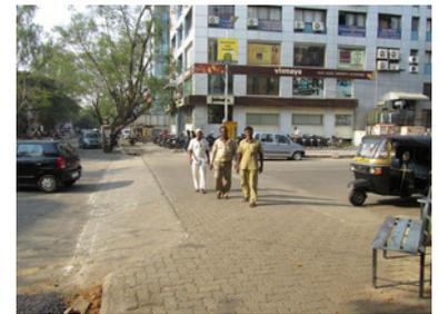
Figure 29.23. At this junction in Pune, India, a raised pedestrian crossing compels drivers to slow down and allows pedestrians to remain at the same level while crossing to the other side. *Chris Kost*
