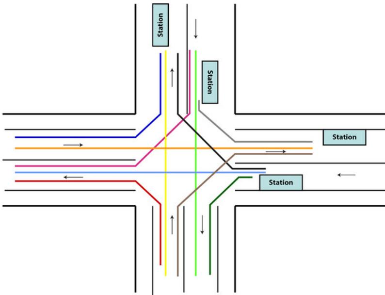
Figure 22.61. An alternative means of connecting split and side-aligned stations is to provide a full set of route permutations. *HHO Africa*.
