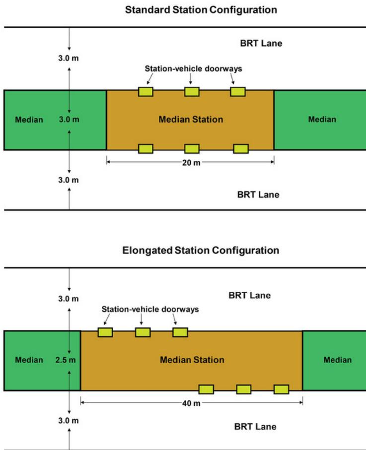
Figure 22.55. Comparison of a standard and elongated station configuration. HHO Africa.
