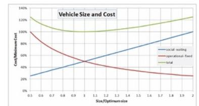
Figure 6.24. The social cost of waiting (blue line) increases and operational costs (red line) decrease as bus size increases. The trick is to balance the two to find the optimum where the sum of costs is minimized. Image *Elebeta*.
