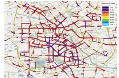
Figure 5.8. Analysis of existing bus speeds for Tianjin, China, BRT. ITDP.
