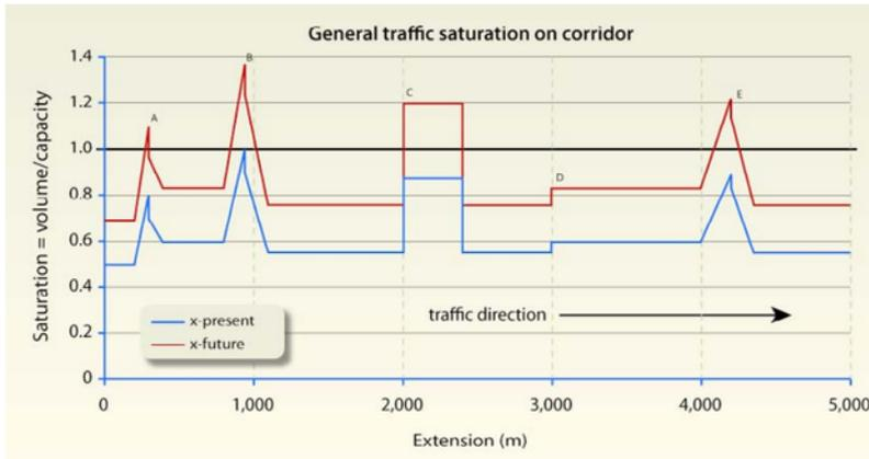
Figure 24.15. Current demand saturation level for mixed traffic can be expected to off-set the transference of one lane to the planned BRT system. *ITDP*.
