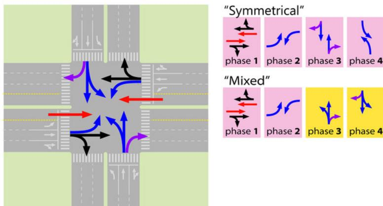
Figure 24.36. With the insertion of BRT (red) in a four-stage signal, the cross-traffic turn from the same direction needs to have its own phase. *Elebeta.*
