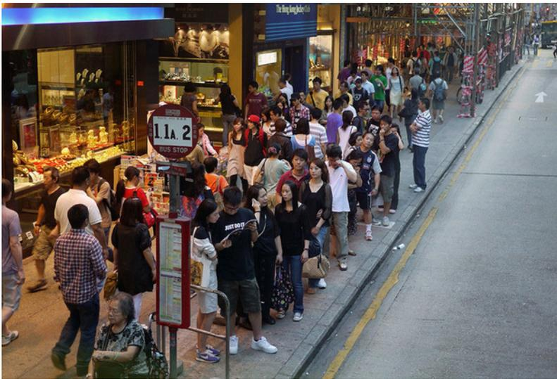
Figure 29.62. The limited capacity of this walkway at a public transport interchange in Hong Kong reduces the pedestrian level of service. *ITDP*
