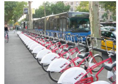
Figure 31.53. Barcelona's bike-share system features sturdy bicycles with internal gearing, fenders, chain guards, and front baskets. *Nelson\Nygaard*.
