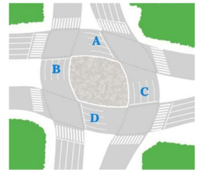
Figure 24.61. In this scenario, the intersection is converted to a roundabout with vehicle queuing areas at points “A,” “B,” “C,” and “D.” The BRT vehicles enter mixed traffic just before the intersection and move through the intersection with a two-phase signal. ITDP.
