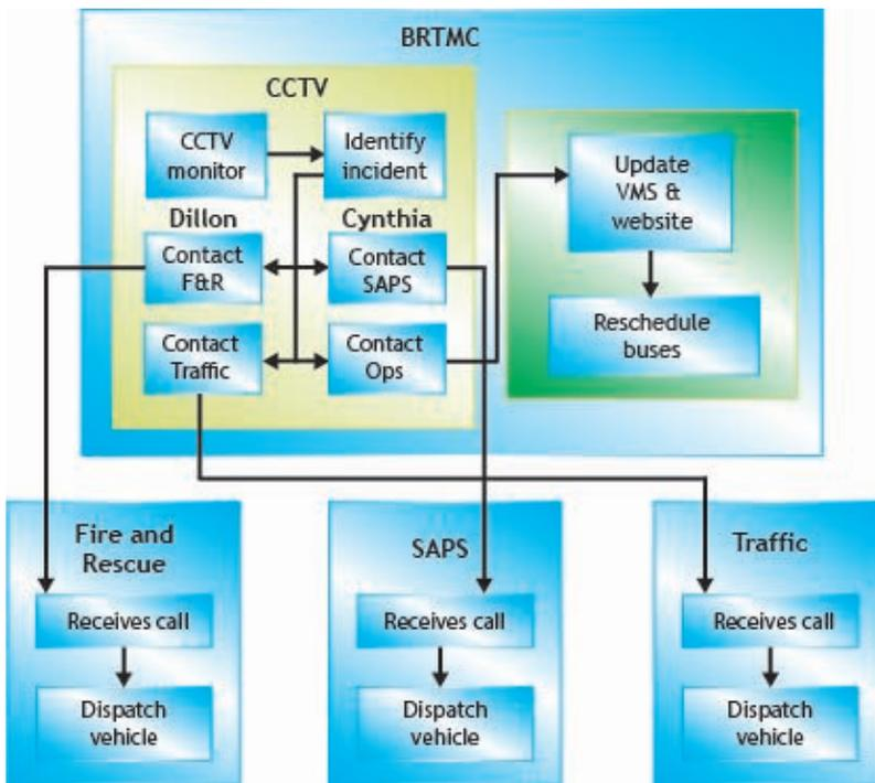
Figure 27.18. Emergency process. TECHSO.
