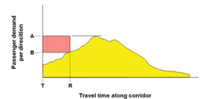
Figure 6.69. Adding a second local service that covers only the highest demand segment of a corridor can reduce operating costs while limiting additional delay for customers. Image Pedro Szász.
