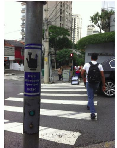
Figure 24.9. As an example of actuation, pedestrians may “call the controller for a service” by pressing a button, as in this crossing in São Paulo. *Jonas Malaco.*
