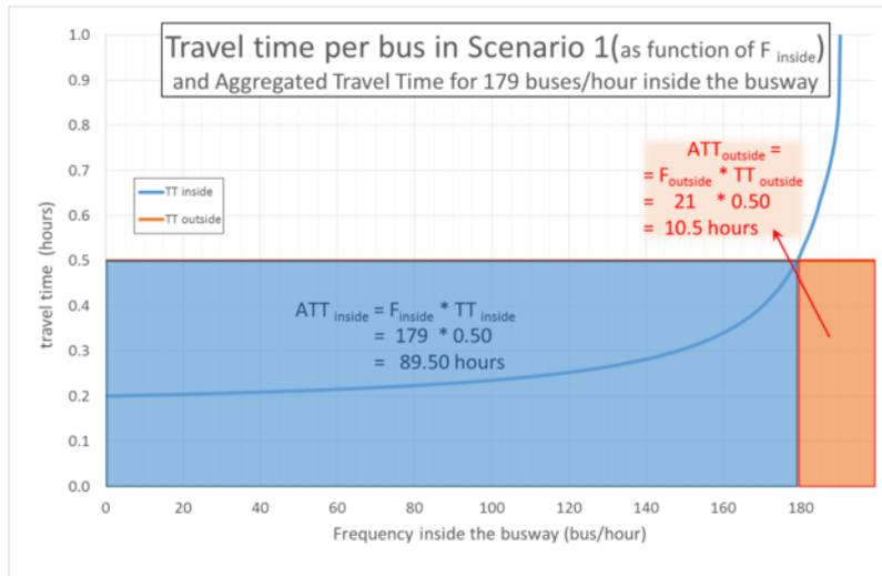
Figure 6.36. Scenario I aggregated travel times, obtained by multiplying by the fixed travel time for all buses (0.5) by the number of buses inside the busway (179, represented by the blue shading) and outside the busway (21, represented by the orange shading), one should get  $ATT_{inside}(F_{inside} = 179) = 89.50$  hours and  $ATT_{outside}(F_{inside} = 179) = 10.5$  hours, respectively. *Elebeta*.
