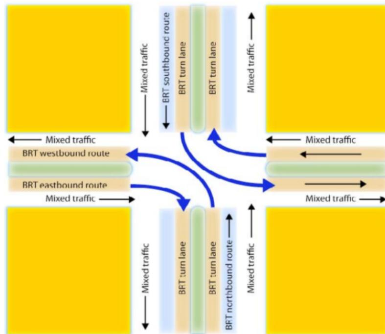
Figure 24.54. Configuration for a system with a fully dedicated BRT turning lane. ITDP.
