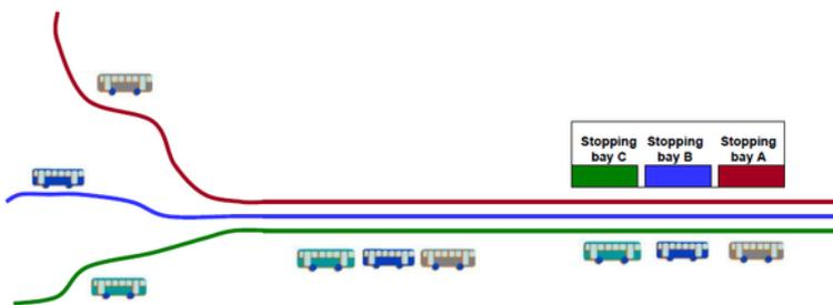
Figure 7.6. Conveying systems order vehicles when entering the corridor, so they ride as "train" and the docking position for every route at the station is fixed, preventing users from running up and down the platform. Pedro Szász.
