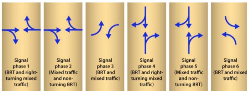
Figure 24.56. To permit a full range of both BRT and mixed-traffic turning movements, six signal phases would be required. *ITDP*.
