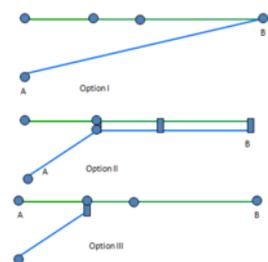
Figure 6.77. Three options for planning routes near a BRT corridor. Image ITDP.
