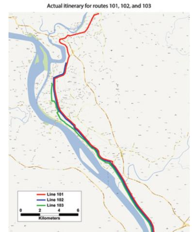
Figure 6.70. Yichang overlapping services can be maintained only in the CBD doubling frequency in the high demand part of the corridor, while limiting total route length to minimize irregularity. ITDP.
