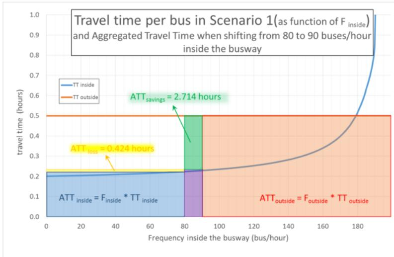
**Figure 6.38.** The losses to the buses inside the busway,  $ATT_{loss}$  as represented by the light yellow rectangle, of shifting 10 buses into the corridor, amount to 0.424 hours. The aggregated time savings of those 10 buses,  $ATT_{savings}$  as represented by the green rectangle, amounts to 2.714 hours. Since the time savings are greater for those 10 buses than the losses to other buses already inside the corridor, it is still beneficial to shift in more buses. *Elebeta.*
