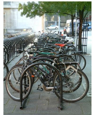
Figure 31.29. A U-shaped bike rack is a low-cost and relatively secure option. *Lloyd Wright.*
