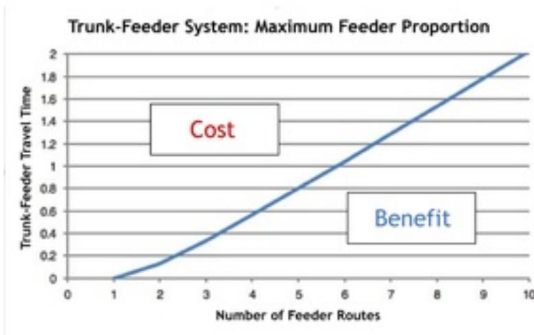
Figure 6.44. Conditions under which benefits can be accrued from vehicle size optimization in a trunk-and-feeder system: The blue line above shows the points at which the benefits and costs of direct services and trunk-and-feeder services are equal, determined by two variables: the proportion of the total trip time that takes place on the feeder route (y axis) and the total number of feeder routes that share the trunk demand (x axis). Image Pedro Szász.
