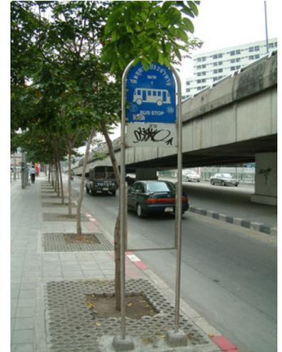
Figure 24.85. While vehicles in mixed traffic can bypass a congested intersection in Bangkok, public transport vehicles are often consigned to serving stations near the intersection. This can result in slow average speeds for public transport. Lloyd Wright.
