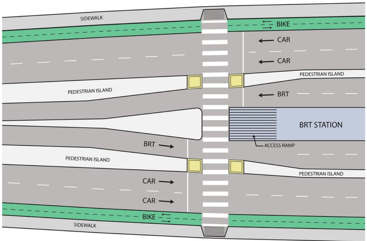
Figure 29.53. Pedestrian islands should be constructed between the busway and mixed traffic lanes. ITDP
