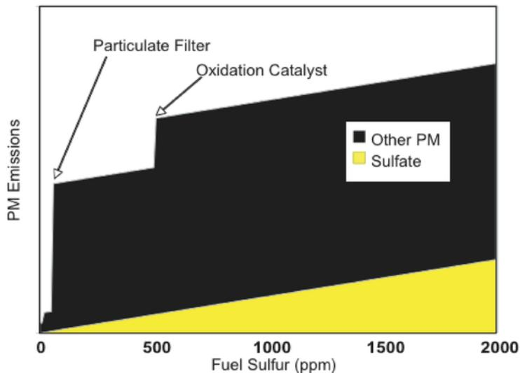
Figure 20.31. There is a close relationship between the emissions of sulfur and emissions of particulate matter (PM).
