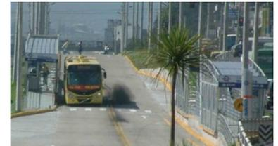
Figure 20.28. On the Quito Central Norte corridor, the Euro III-compliant vehicles are not producing the desired results due to the use of 500 parts per million of sulfur in diesel fuel. Lloyd Wright
