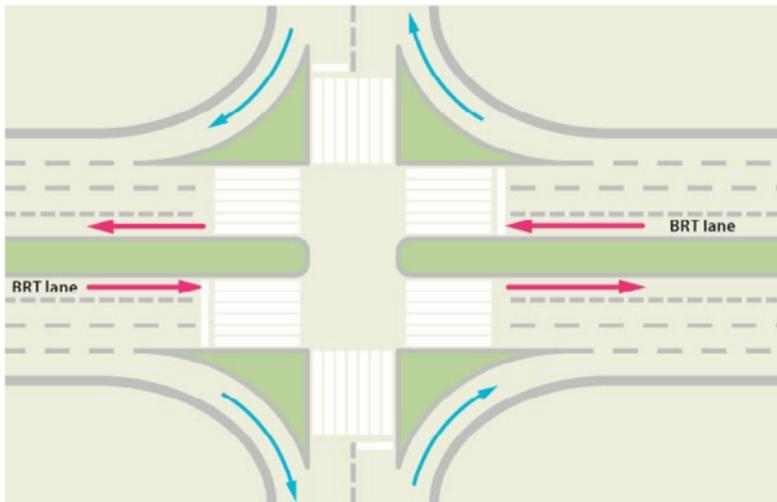
Figure 24.70. The introduction of a pedestrian island between the curbside-turn lane and the crossing can significantly help pedestrians safely cross within the standard two-phase traffic signal. *ITDP.*
