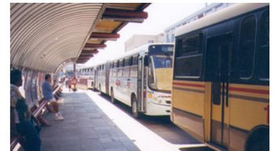
Figure 7.18. Convoying allows the Porto Alegre system to achieve peak capacities of over 20,000 pphpd, but at the same time this technique can result in busway and station congestion, and therefore slow average vehicle speeds. Lloyd Wright.
