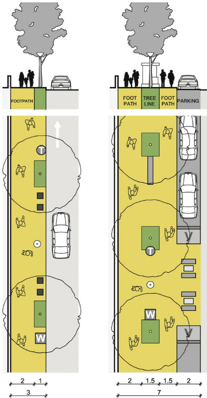
Figure 29.18. The smallest well-functioning footpath/tree package has a width of 3 meters, including a 2-meter clear space and 1-meter tree pits. Street furniture is positioned in line with the tree pits to maintain 2 meters of clear space. Wider footpaths can accommodate street vending and larger seating areas, and are recommended in areas with large pedestrian volumes. Diagram courtesy of ITDP's *Better Streets, Better Cities* (2011)
