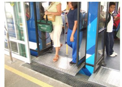
Figure 7.23. Even bus approach to station being faster, using boarding bridges, as seen here in Guayaquil, Ecuador, usually increases dead time, while certainly decreases boarding time per passenger. Lloyd Wright.
