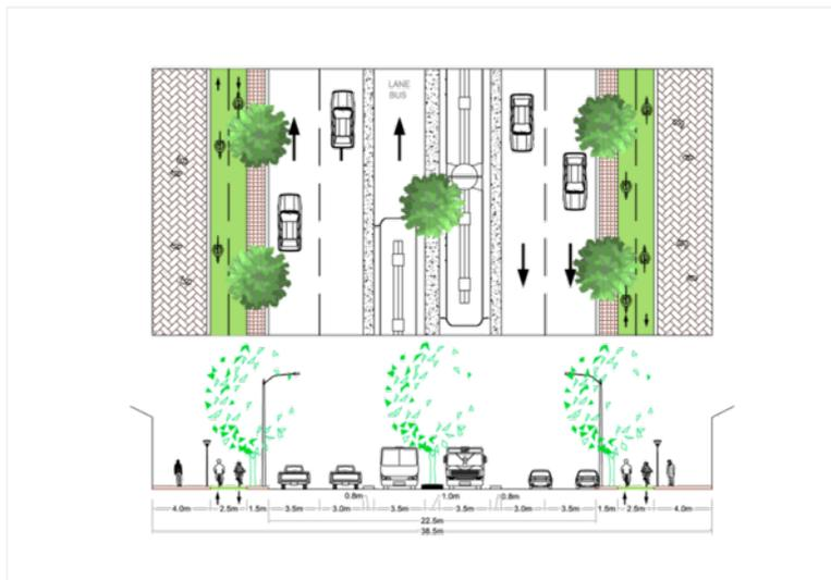
Figure 22.17. Plan and section view of Stretch 5 at a width of 38.5 meters. *Logit.*
