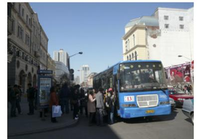
Figure 7.25. On-board fare collection and fare verification dramatically slows customer throughputs, as evidenced here in Harbin, China. Photo Lloyd Wright.
