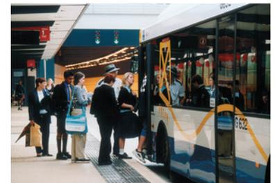
Figure 20.11. Low-floor vehicles without platform-level entry and pre-board fare verification can result in longer dwell times and not actually provide access to the physically disabled, as shown in this images from Brisbane, Australia Queensland Transport.
