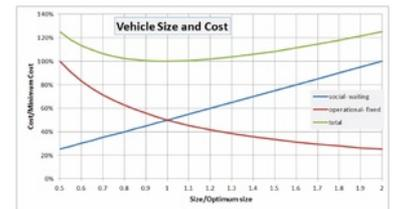
Figure 6.24. The social cost of waiting (blue line) increases and operational costs (red line) decrease as bus size increases. The trick is to balance the two to find the optimum where the sum of costs is minimized. Image *Elebeta*.
