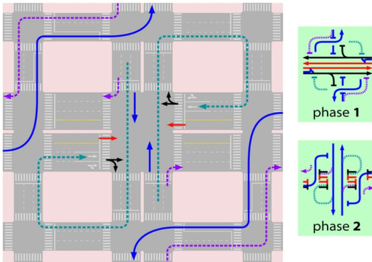
Figure 24.40. It is possible to provide a two-phase coordination for detouring cross-side turns to leave the road upstream and return downstream of the main intersection; additional synchronized traffic lights are required. *Elebeta.*
