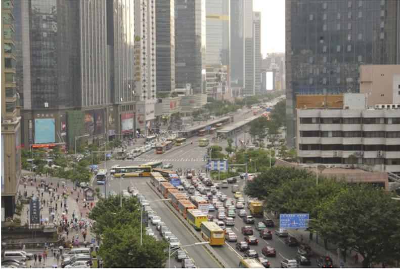
Figure 22.1. Guangzhou, China, is a median-aligned busway configuration with split stations located along the outside of the busway. *ITDP*
