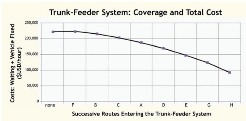
Figure 6.49. Likely total system cost curve if there are many feeder routes and the feeders only constitute a short portion of total trip time. Graph *Pedro Szász*.
