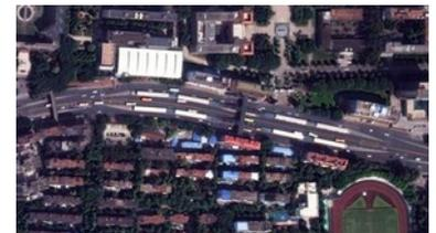
Figure 6.57. On the Guangzhou BRT, the highest capacity direct service BRT system in the world, there are stations with up to four sub-stops and twelve docking bays (two to three docking bays per sub stop) per direction. Image Bing Maps.
