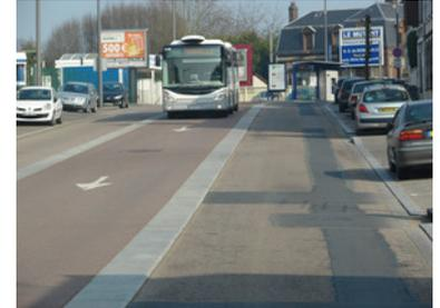
Figure 22.43. The virtual lane concept in Rouen, France, where a single centrally located bus lane is used to provide bus priority in both directions of travel. *Andre Frieslaar.*
