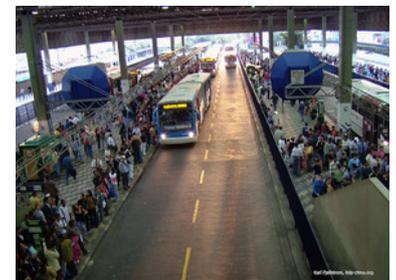
Figure 6.19. Passing lanes prevent queue formation at stations in São Paulo, deliver significant travel time savings to customers. Karl Fjellstrom, *ITDP China*.
