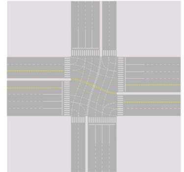
Figure 24.28. Exchanging width between entrance and exit sections where turning volumes are high enough to allow the change to improve capacity meaningfully. *Elebeta.*
