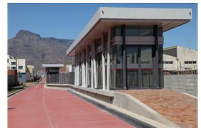
Figure 22.56. An off-set station in Cape Town, South Africa. The platforms are arranged a distance apart to allow for a passing lane on each side at the station docking area. ITDP.
