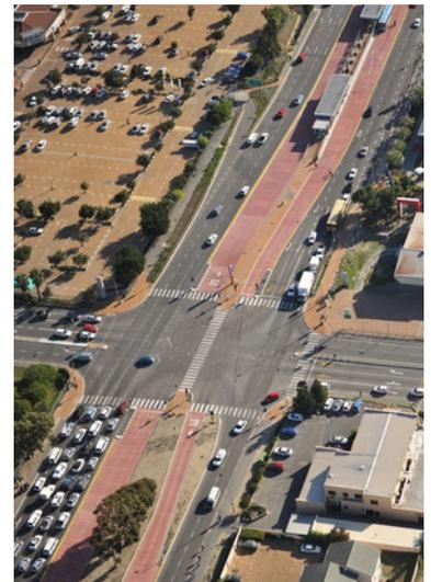
Figure 24.29. Cape Town, South Africa's standard four-phase intersection with a cross-traffic-turn waiting area using the narrowed width of the opposite way. *Bruce Sutherland.*
