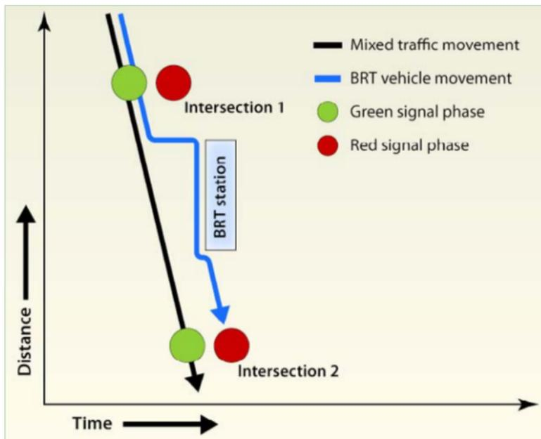
Figure 24.33. Coordination for mixed traffic does not help the BRT corridor when there is a station between intersections. If the green time of the green wave has the same length of total dwell time at stations, the effect can be particularly harmful, as it increases the chances that the BRT vehicle's arrival at an intersection after a station will be during the red time. *ITDP.*
