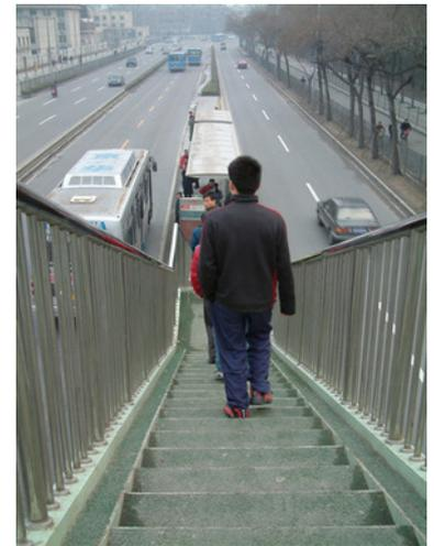
Figure 29.37. A steep, narrow stairway in Beijing makes for poor accessibility to the busway. *Lloyd Wright*
