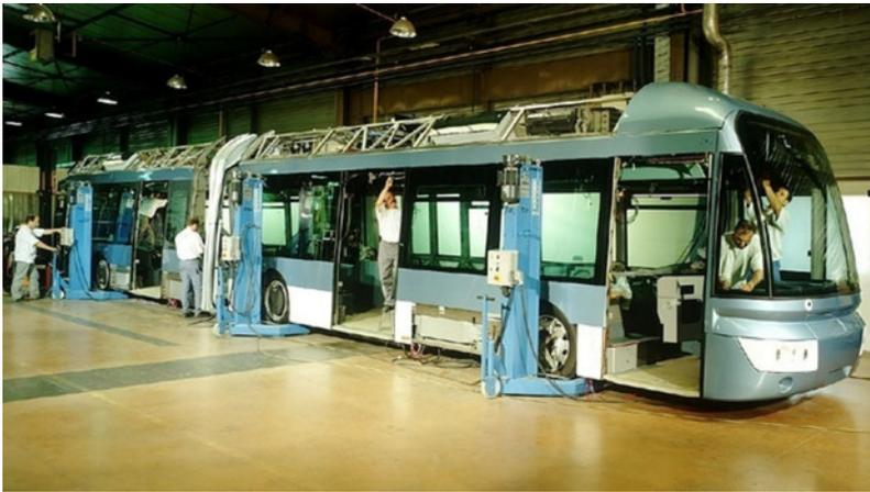
Figure 20.47. Specialized manufacturing of low-volume vehicles can dramatically increase overall costs. TCRP BRT image library.
