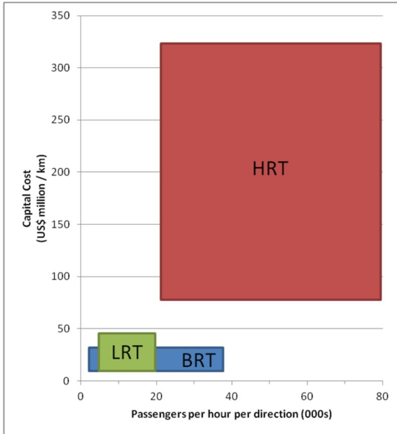
Figure 2.12. Passenger throughputs and capital cost for mass transit options. This figure compares the range of passenger throughputs for each technology measured against the range of capital costs. The ranges presented in Figure 2.12 are based on observed, not theoretical, data (Tables 2.8 and 2.9). *ITDP*.
