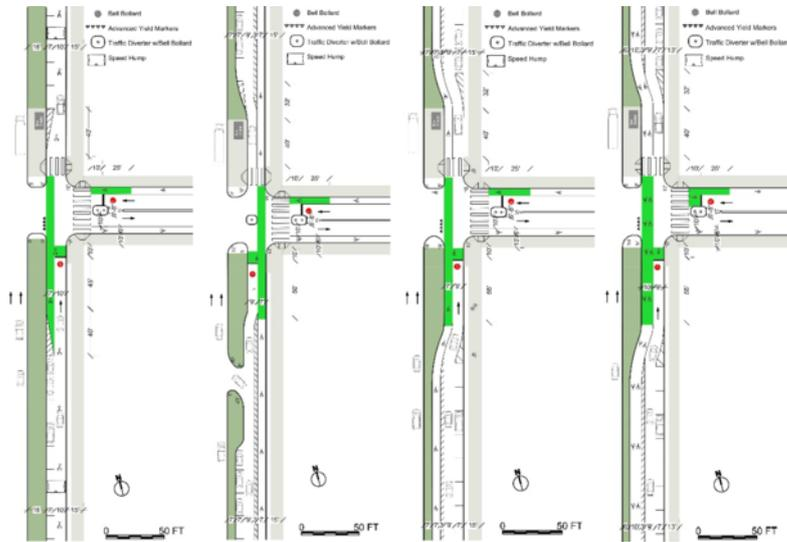
Figure 31.13. Plan view of four options for locating bicycle facilities in the service road of a multi-way boulevard (from left): bike lane only at intersections; bike lane on right side; bike lane on left side against median; and two-way bike lane on left side against median. *Nelson\Nygaard.*
