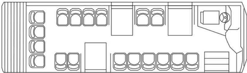
Figure 20.17. Example of customer configuration for a short vehicle. ITDP
