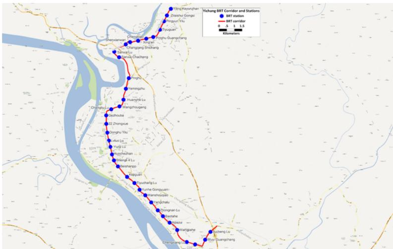
Figure 25.50. The high capacity BRT system in Yichang, with larger stations, averages 645 meters between stations. ITDP-China.
