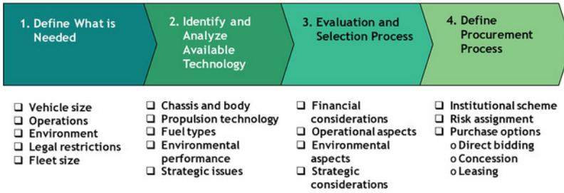
Figure 20.2. Decision-making process for vehicle selection. *ITDP*
