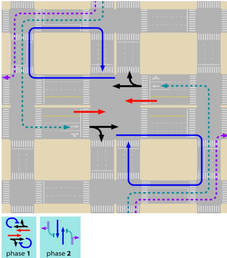
Figure 24.39. Three curbside turns after crossing the intersection is a simple alternative to eliminating cross-traffic turns; despite crossing the intersection twice, it does not create much conflict with existing flows. *Elebeta*.
