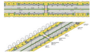
Figure 29.22. Formal pedestrian crossings, in which pedestrians remain at the same level as the footpath (e.g., +150 millimeters), and vehicles pass over ramps are required on major streets. Between formal crossings, landscaped pedestrian refuge islands should be provided at intervals of approximately 50 meters. At both formal and informal crossings, curb extensions into the parking lane reduce the total crossing distance. *ITDP's Better Streets, Better Cities (2011)*
