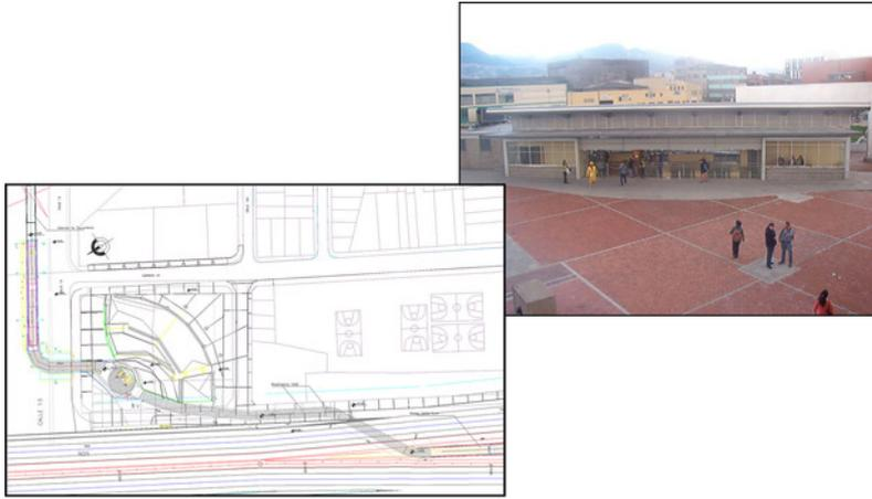
**Figure 25.3.** A schematic and external view of the Ricaurte interchange station in Bogotá where customers walk through a pedestrian tunnel to access the different corridors. The Ricaurte station also includes customer amenities such as restrooms, an information centre, and quality public space. *ITDP.*
