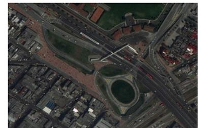
Figure 24.90. At the major intersection of TransMilenio's Calle 80 corridor and NQS corridor is a set of underpasses and an overpass link to the exclusive BRT roundabout. *Google Earth*.
