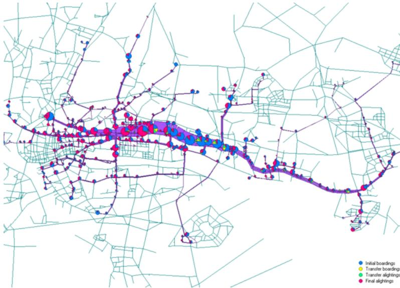
Figure 4.15. Aggregate data for boarding and alighting at current bus stops, allocated to future Guangzhou BRT stations (passengers per hour) in May 2009. (The system opened in February 2010.) ITDP.
