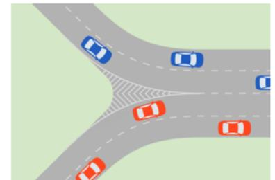
**Figure 24.2.** A channeled Y junction without conflicts does not have the basic element that defines an intersection. *Elebeta.*
