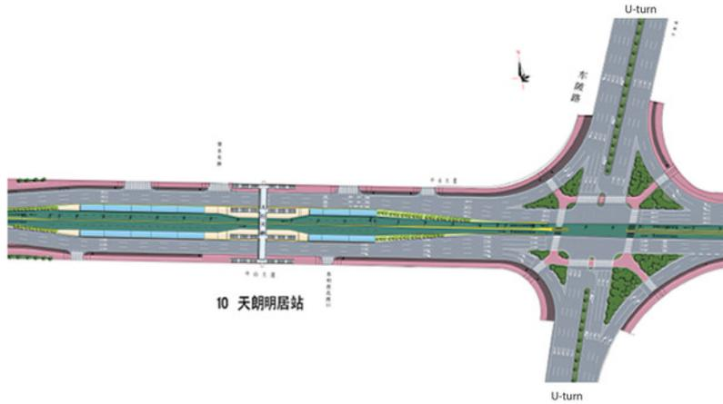
Figure 24.14. The same intersection as depicted in Figure 24.13 on a BRT corridor in Guangzhou, China. The station is located away from the intersection of the BRT corridor and Chibei Avenue. In order to turn across traffic, the two-phase intersection requires a U-turn in the perpendicular road. Before the BRT, this four-phase intersection was a major traffic-congestion point. *ITDP and GMEDRI.*
