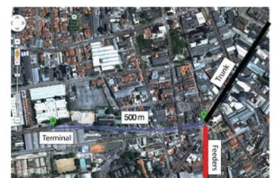
Figure 6.56. Trunk-and-feeder terminal Santo Amaro in São Paulo is poorly located and accesses are poorly designed, causing additional travel times. Image Arthur Szász.
