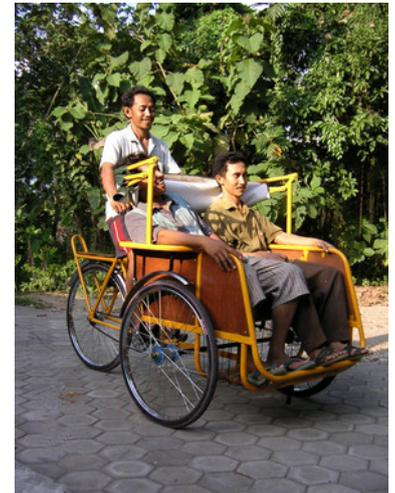
Figure 31.60. The redesigned Indonesian becak is lighter and more stable than traditional models. *ITDP*.
