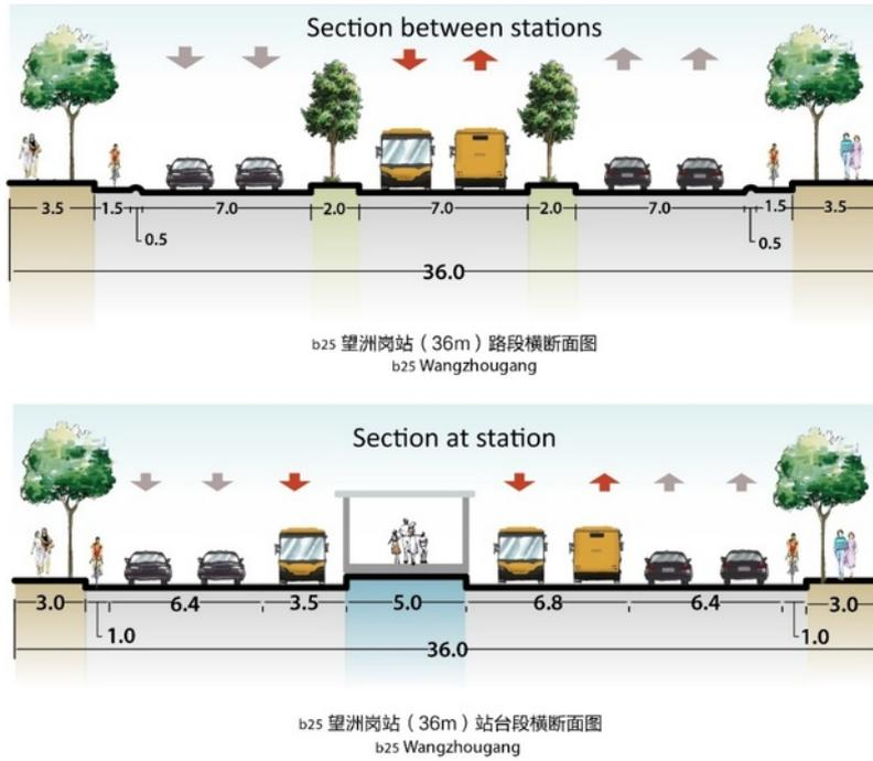
Figure 25.57. Cross-section at and between stations at Wangzhougang BRT station in Yichang. ITDP
