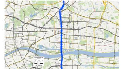
Figure 5.7. Bus flows of all routes in Guangzhou Avenue (being considered for BRT implementation) in Guangzhou, China. Peak points in the proposed north-south BRT corridor (in blue) have more than two hundred buses per hour in a single direction. Peak points in off-corridor locations, showing where the Guangzhou Avenue routes operate, feature more than 150 buses per hour in a single direction. ITDP.
