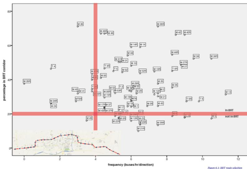
Figure 4.20. Peak frequency and percentage of route traversing the corridor. Example of BRT route selection in a proposed BRT corridor in Ulaanbaatar, Mongolia. Image *ITDP*.
