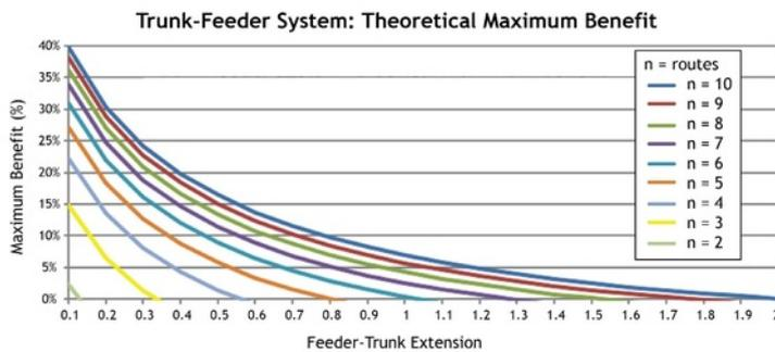
Figure 6.45. Range of possible benefits from vehicle size optimization from for trunk-and-feeder systems, depending on the number of routes (each line) and the share of the total trip time accounted for by the feeder route (x axis). Pedro Szász.
