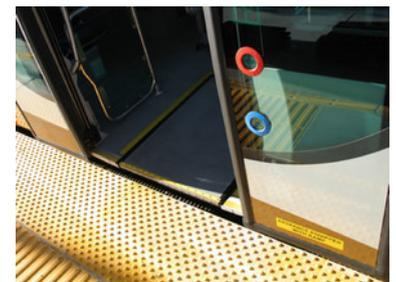
Figure 7.31. When operating properly, the optical guidance system employed in Las Vegas, Nevada, USA, can align the vehicle within a few centimeters of the platform. NBRTI.
