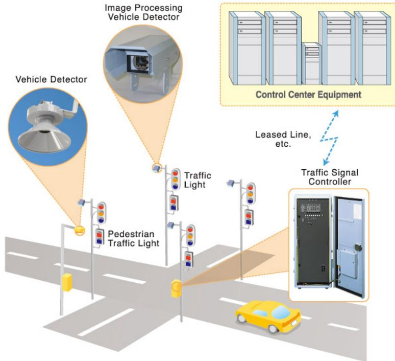
Figure 19.9. Signal control system. Sumitomo Electric.
