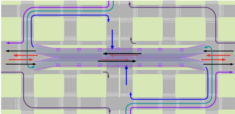
Figure 24.88. Curbside detour for perpendicular flows above the flyover. *Elebeta*.
