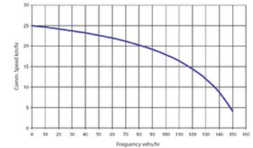
Figure 6.23. Service frequency and the potential impact on vehicle speed at a station with no passing lanes. Graph Steer Davies Gleave.
