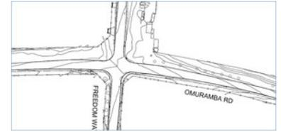
Figure 23.3. Typical output from a topographical survey HHO Africa.
