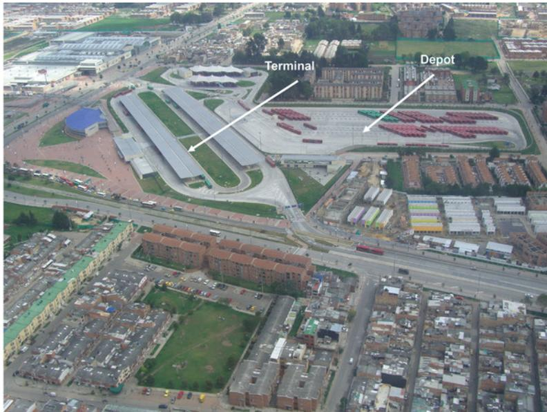
Figure 26.1. In Bogotá, most depots are located next to the terminal areas in order to improve operational efficiency. Oscar Diaz and Por el País que Queremos (PPO).
