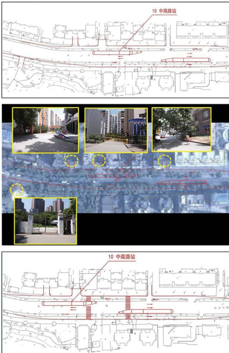
Figure 29.55. This series of images from Yichang, China, shows how a BRT station location is slightly adjusted to better serve the surrounding pedestrian network. The top image shows the initial layout. The second image locates adjacent streets and crossing opportunities. In the last image, the station has been moved to the left and crosswalks added. *ITDP*
