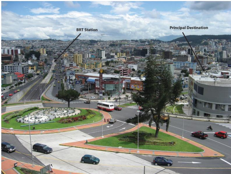
Figure 24.74. In the case of Quito's Central Norte line, the presence of a BRT underpass has meant that the closest station to a key destination, the Plaza of Américas commercial center, is several hundred meters away. Lloyd Wright.
