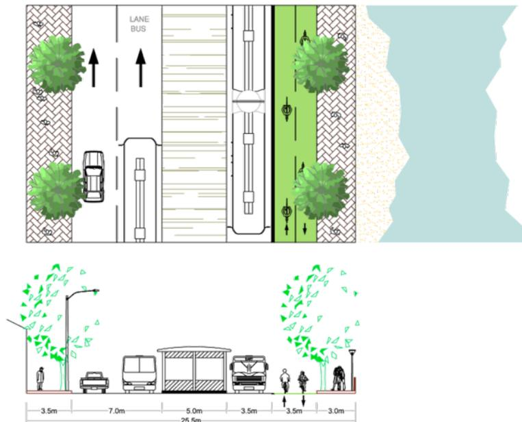
Figure 22.14. Plan and section view of Stretch 1 at a width of 25.5 meters. *Logit.*
