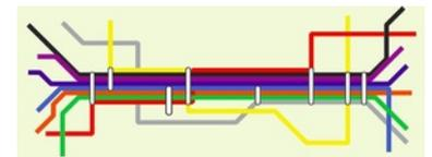
Figure 2.10. This diagram of direct services shows how multiple routes that operate along a single corridor can go to different destinations, reducing door-to-door travel times. ITDP.
