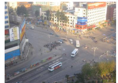
Figure 24.57. In Kunming, turning BRT vehicles leave the busway and enter a mixed-traffic lane to finalize the turning movement. *ITDP*.
