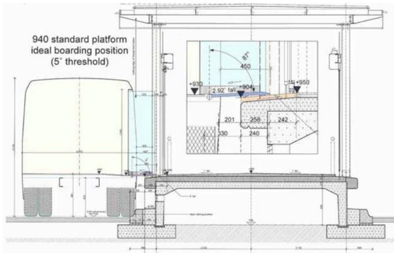
Figure 30.45. Diagram providing detail of the alignment of the boarding bridge with the platform. City of Cape Town.
