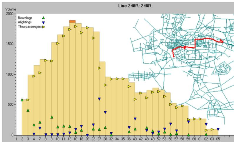
Figure 6.20. Output of a boarding and alighting survey for bus route 248R in Guangzhou, China, during the peak hour. The “Critical Link” is between Stop 13 and Stop 16. Graph *ITDP*.
