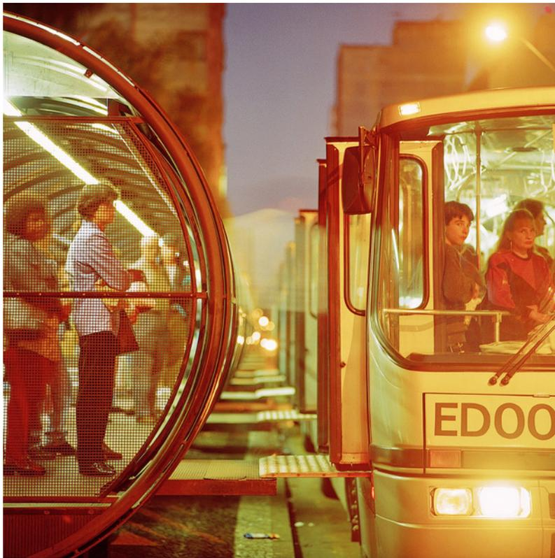
Figure 7.22. System in Curitiba, Brazil, utilize a boarding bridge between the vehicle and platform to facilitate easy boarding Volvo
