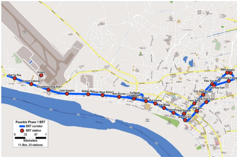
Figure 25.49. The proposed medium capacity BRT system in Vientiane averages one station every 500 meters. ITDP-China.
