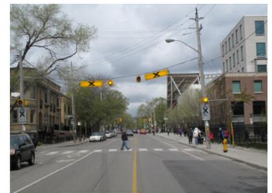
Figure 29.43. Example in Toronto of a pedestrian crosswalk with vertical elements indicating to drivers the location of the crosswalk. *Michael King*
