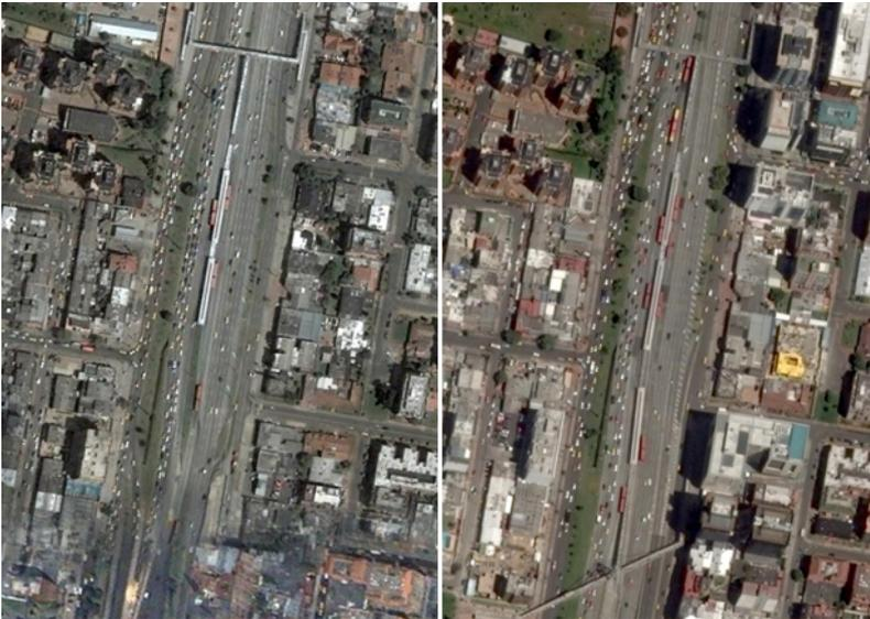
Figure 25.35. The image on the left is the Calle 100 station in 2005 with just two sub-stops, but space for more. The image on the right is the same station in 2013 with an additional sub-stop having been added due to increased demand. *Google Earth.*
