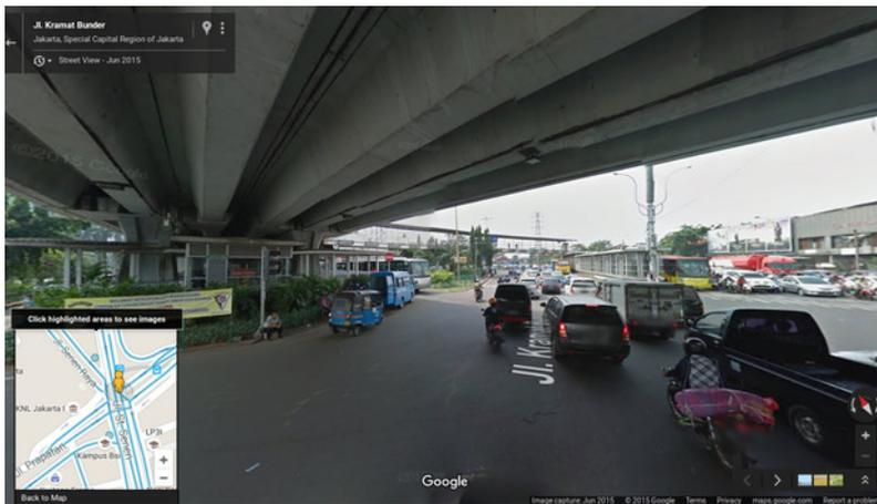
Figure 24.86. This five-leg intersection under the Senen Street flyover in Jakarta has several forbidden turns; the intersection of two BRT corridors and a four phase-signal causes delays in both corridors and is even worse than mixed traffic. Google Maps.
