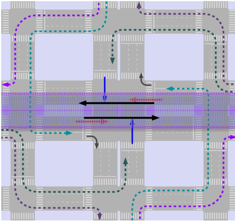
Figure 24.87. Curbside detour for perpendicular flows under the flyover. *Elebeta*.
