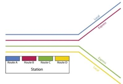
Figure 7.33. Platform order based on service clustering. Image ITDP.
