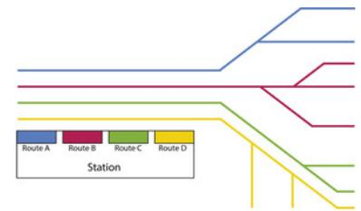
Figure 7.32. Platform order based on geographic proximity of routes. Image ITDP.
