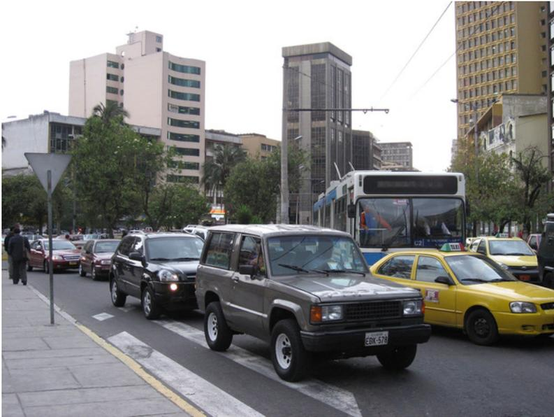
Figure 22.23. In this image from Quito, Ecuador, the Trolé BRT vehicle operates in an “exclusive” curbside lane, but is blocked by merging traffic from a side street. A median busway would largely avoid these types of conflicts. Lloyd Wright.
