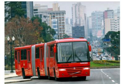
Figure 20.3. In Curitiba, 24-meter bi-articulated vehicles are utilized on trunk corridors. Volvo Bus Corporation.
