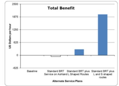
Figure 6.74. Total estimated benefits for four alternative service plans based on modeled results on Chicago’s Ashland corridor: Existing services (baseline), the initial proposal for eliminated stops along Ashland, a service scenario where two additional routes with direct services to the CBD have been added, and a final service scenario where “S” shaped routes have been added. Image Pedro Szász.
