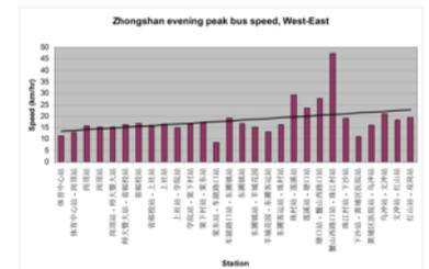
Figure 4.21. Using the same boarding and alighting survey, average vehicle speeds in the corridor can be calculated and arranged in a graph. *ITDP*.
