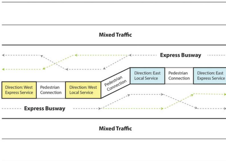
Figure 22.57. By offsetting the sub-stops and elongating the platform, passing lanes can fit into relatively narrow road widths. *Lloyd Wright.*
