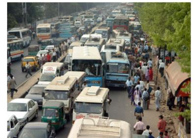
Figure 5.25. An exclusive busway on the road in Bangladesh would likely make mixed traffic less congested because of the high number of buses in mixed traffic. Karl Fjellstrom.
