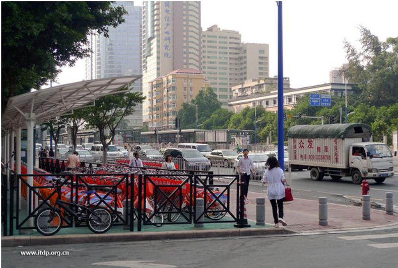
Figure 31.48. An overflow corral at a Guangzhou, China, bike-share station is managed by an attendant, to ensure that empty docks and bicycles are available at peak periods. *ITDP*.
