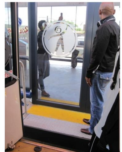
Figure 25.86. In Johannesburg, the sliding door malfunctioned and did not open as the bus pulled up, leaving the passenger stranded between the bus and station. The station attendant quickly came to manually open the doors with a remote control. *ITDP*
