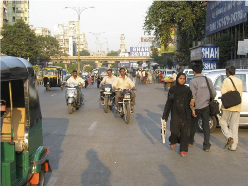
Figure 29.31. However, on arterial streets where motor vehicle speeds are high, and there are no designs aimed at speed reduction; these ad hoc "shared space" arrangements are unsafe and inconvenient for pedestrians. *ITDP*
