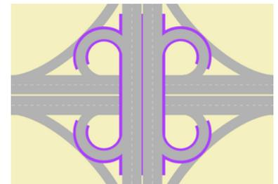
**Figure 24.3.** Separated-grade solutions can eliminate intersections. *Elebeta.*
