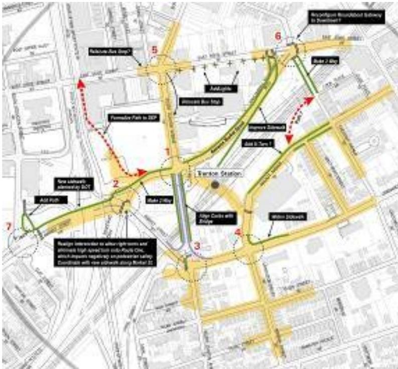
Figure 28.32. An analysis of actual five-minute walking distances around station, Trenton, New Jersey, USA. By identifying actual walking routes the implementing agency could then make upgrades. *NelsonWygard.*
