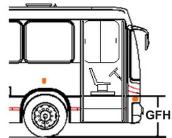
Figure 20.7. GFH 960 mm maximum Long Bus; Rear Engine High Floor ITDP
