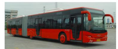
Figure 7.10. The 18-meter articulated vehicle has become standard in many BRT applications. Image of Hangzhou, China, BRT vehicle Kangming Xu (<http://www.brchina.org>).
