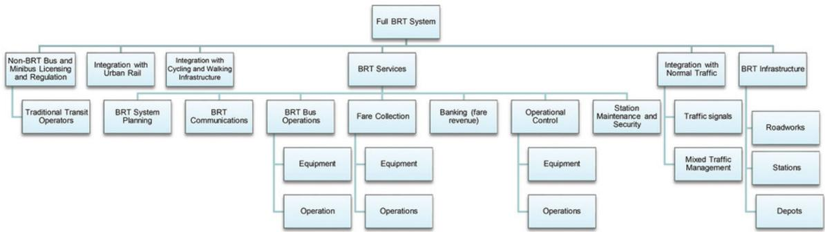
Figure 12.1. Basic functions of a full BRT system. Walter Hook, BRT Planning International, LLC.
