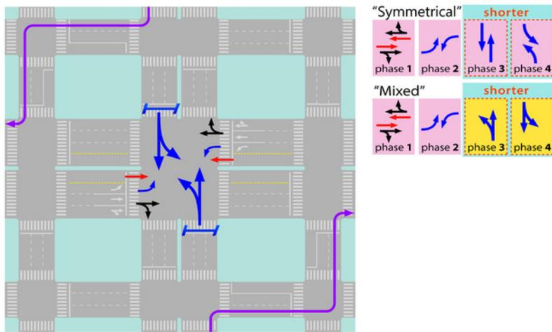
Figure 24.37. Curbside-turn detour can leave width in the main intersection available to crossing flows. *Elebeta.*
