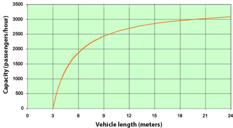
Figure 7.11. Relationship between vehicle size and capacity. Graph Steer Davies Greer.
