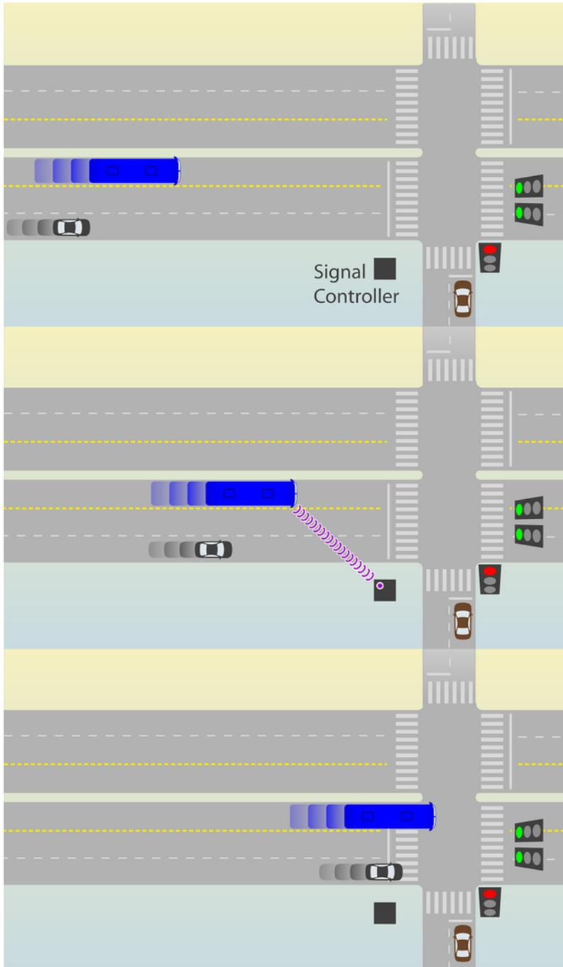
Figure 24.19. Using active priority, the green time for the BRT corridor is extended when a BRT vehicle is detected approaching the intersection. *ITDP*
