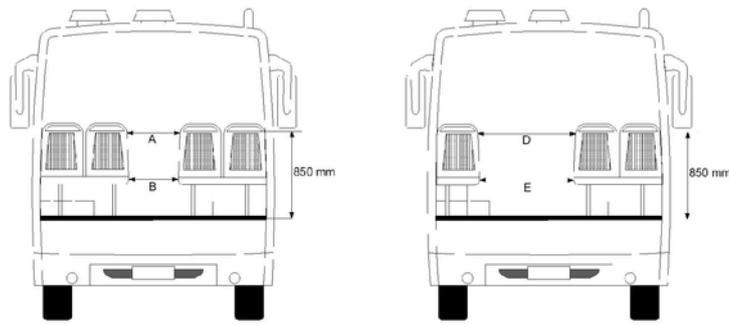
Figure 20.19. The aisle located between the doors in all types of vehicles must not have double seats on both sides. ITDP
