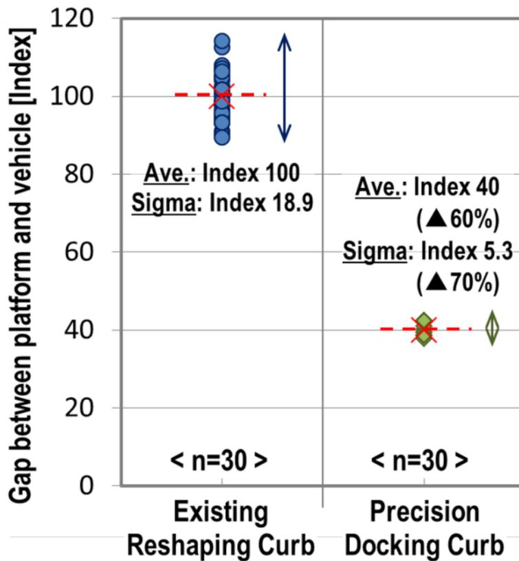
Figure 25.97. The gap improvement from using the precision docking curb method. *Bridgestone*
