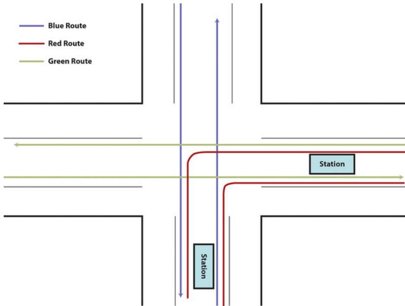
Figure 22.62. However, the required number of permutations becomes excessive, even for just a single intersection. Median stations permit easier platform transfers and multiple route permutations. *HHO Africa*.
