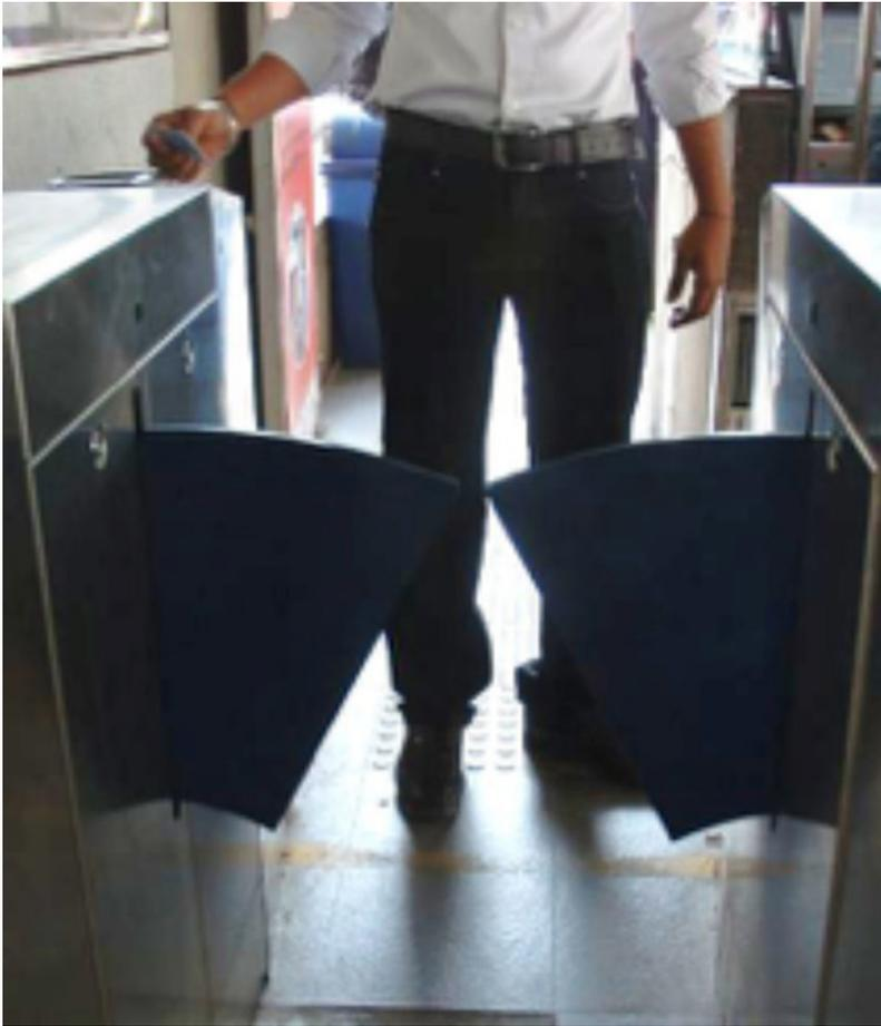
Figure 19.8. Off-board smartcard reader ITDP
