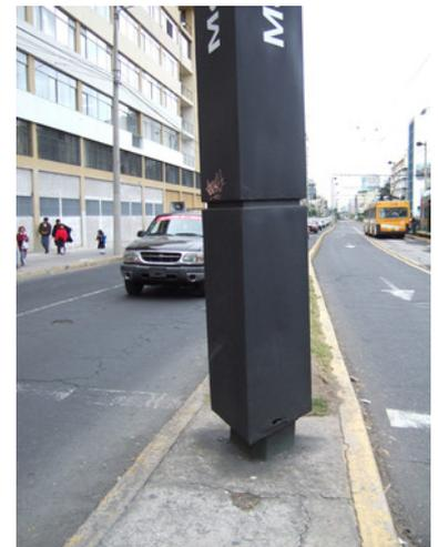
Figure 29.48. This BRT-identification post in Quito is placed in a pedestrian island, and acts to block the pedestrian's view of both oncoming mixed traffic as well as oncoming BRT vehicles. *Lloyd Wright*
