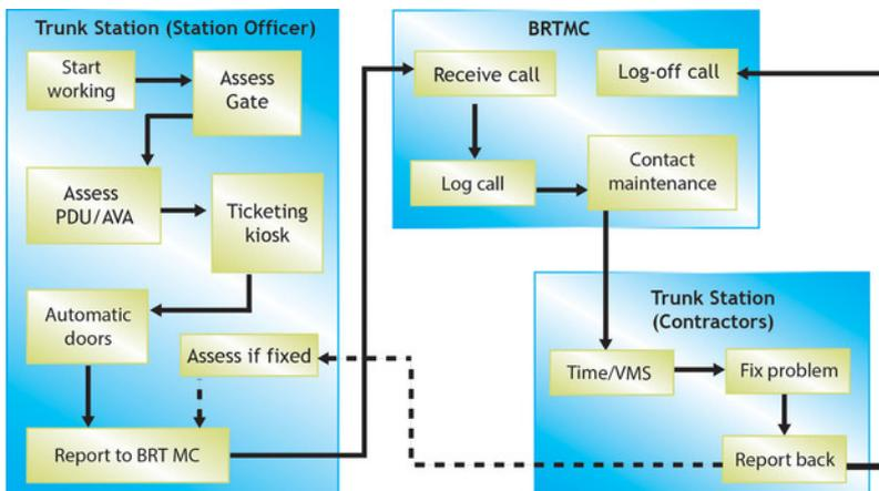
Figure 27.17. Maintenance process. *TECHSO.*
