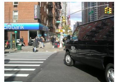
Figure 29.29. Vehicle phase of a leading pedestrian interval in New York City in which vehicles are given a green light only after pedestrians are allowed to begin crossing *Michael King*
