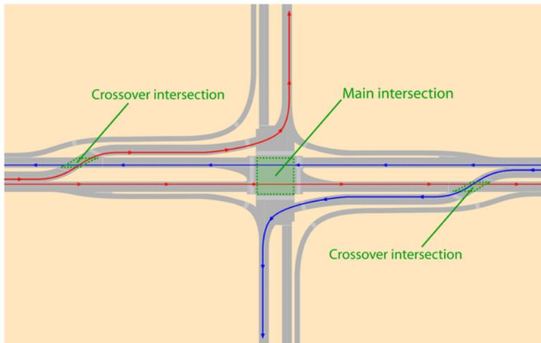
Figure 24.41. In the United States, the concept of previous turn is applied in a less dense urban context by the name of “displaced left turn” intersection. *Elebeta.*
