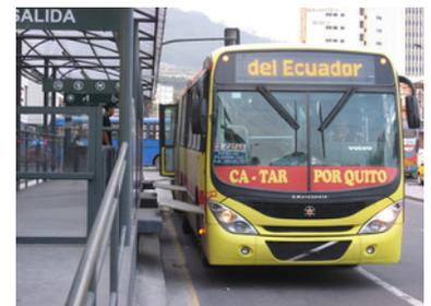
Figure 7.24. The presence of the boarding bridge means that the driver does not need to be as precise docking at the platform. In turn, this can significantly reduce the time lost at stations. Image Lloyd Wright.
