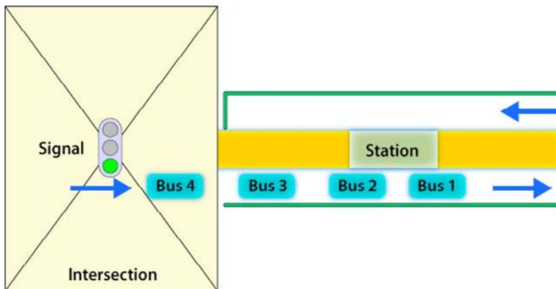
Figure 24.26. For the direction of the BRT system that stops after the intersection, there is a risk that vehicles create a backup into the intersection and block traffic. *ITDP*.
