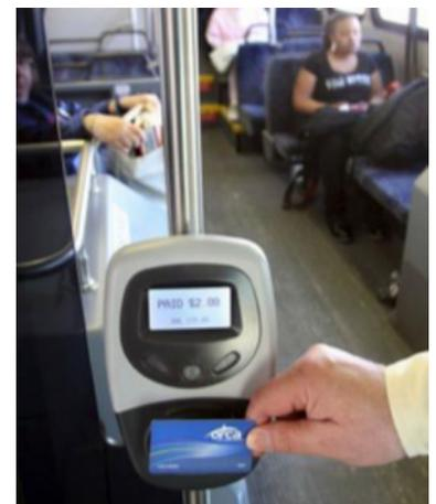
Figure 19.7. Onboard smartcard reader. ITDP
