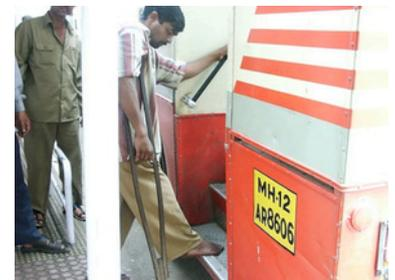
**Figure 30.61.** A low first step makes boarding easier. The man is stepping into the vehicle without lifting his body or bending his knee. Once within the stairwell, he is then better able to use his upper body strength to mount the remaining stairs. *TRL Ltd.*
