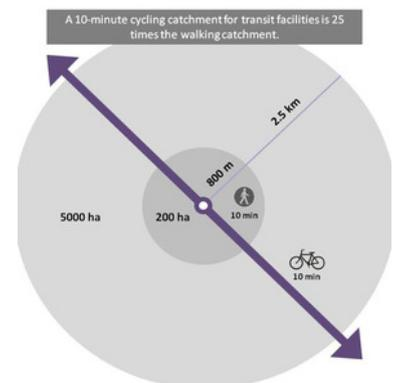
Figure 31.2. Cycling catchment area compared to walking catchment area. *TransLink*
