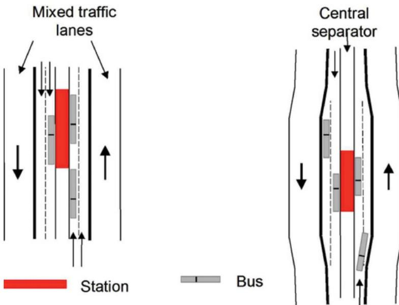
Figure 22.52. Options for provision of a passing lane. *ITDP.*
