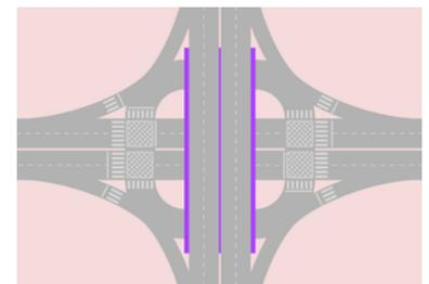
**Figure 24.4.** Depending on space restrictions, separated-grade solutions may not eliminate intersections. *Elebeta.*
