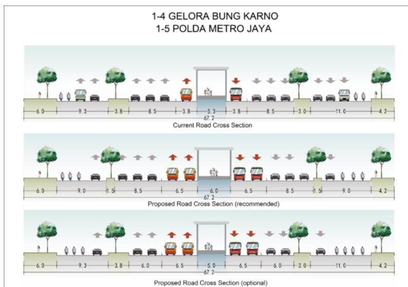
Figure 21.1. Conceptual layout and cross section of a median BRT in Jakarta, Indonesia, to illustrate the insertion of dedicated infrastructure within a corridor. ITDP.
