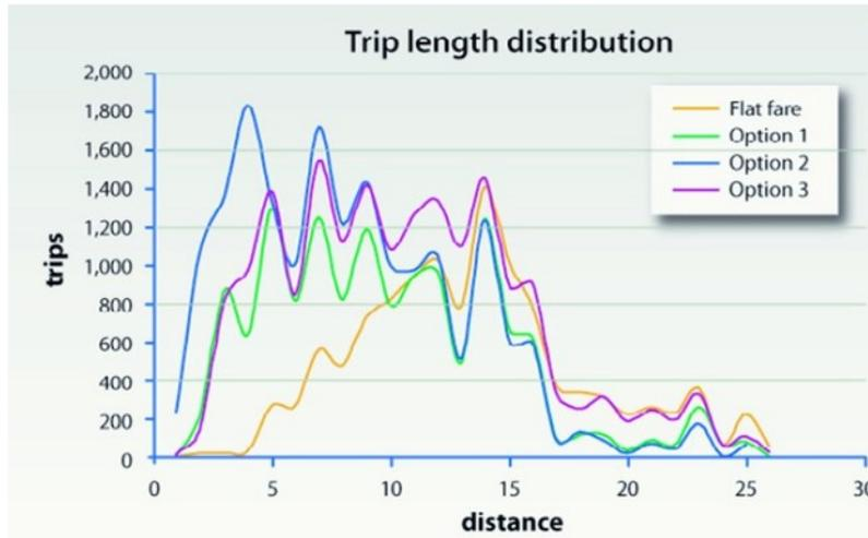
Figure 15.4. Analysis of the impact of different fare structures on Transjakarta's Phase II ridership. ITDP.
