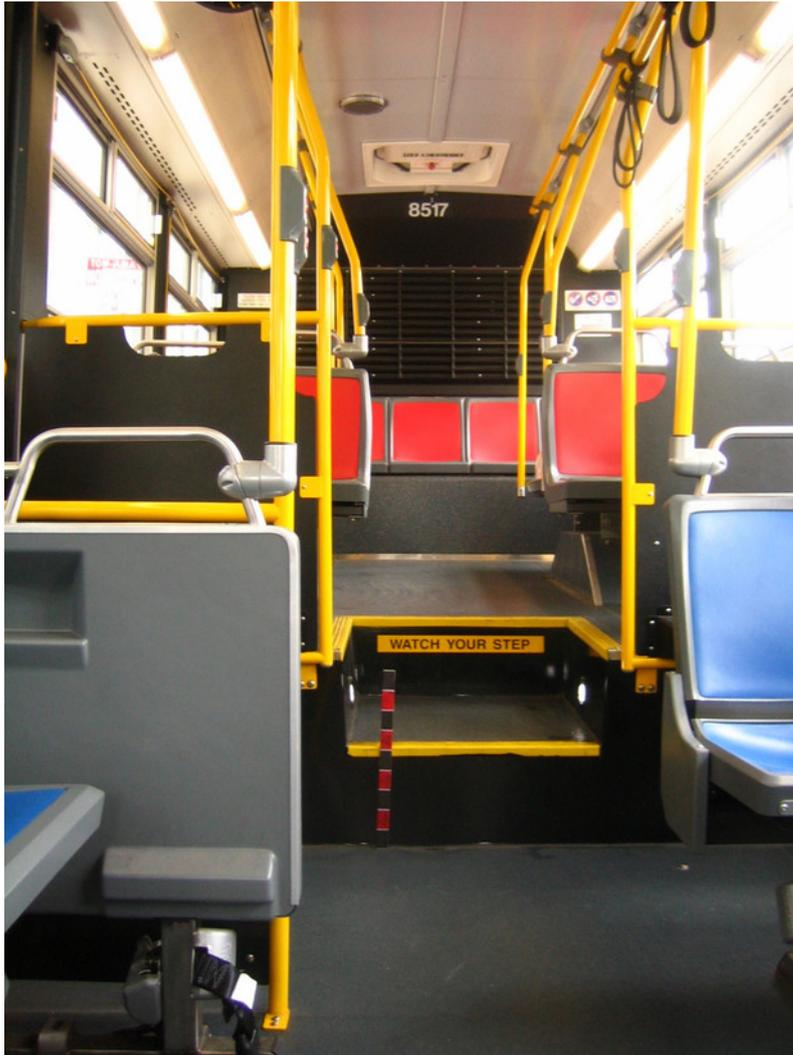
Figure 30.52. Irregular stairs to the rear of the vehicle reduce internal accessibility. *Tom Rickert/AEI.*
