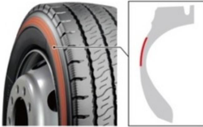
Figure 25.96. The tire reside technology reinforces the side of the tire that rubs against the curb without adding extra weight to the tire and making the tire last 25 percent longer than a conventional tire. No color on the tire – color in image is for illustration. *Bridgestone*.
