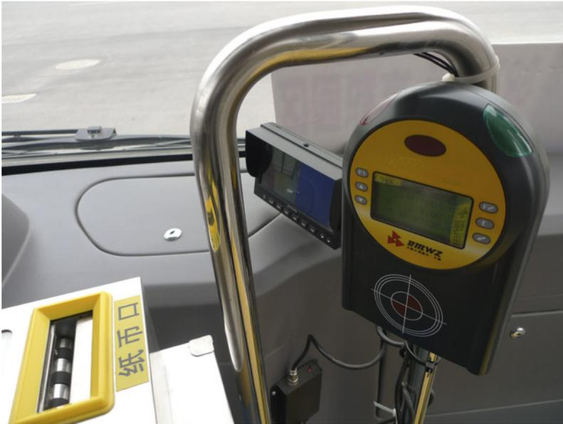
**Figure 18.2.** Onboard fare collection on a feeder bus in Yancheng, China, allows customers to connect to the BRT using a smart card payment system. *Liu Henian.*
