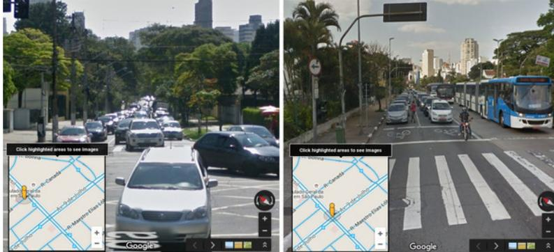
Figure 24.47. Auxiliary street (left) has higher mixed-traffic capacity than the main corridor (right) in São Paulo. Google Maps.
