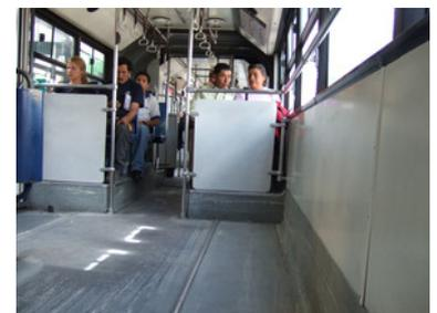
Figure 20.24. Space allocated for special-needs customers, such as those with wheelchairs, can also be useful in meeting standing capacity during peak periods. *Lloyd Wright*.
