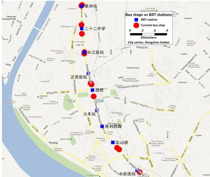
Figure 25.52. Current bus stops and proposed BRT stations by ITDP-China in the Yichang center area. ITDP-China.
