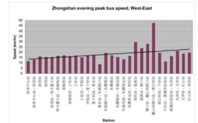
Figure 4.21. Using the same boarding and alighting survey, average vehicle speeds in the corridor can be calculated and arranged in a graph. *ITDP*.
