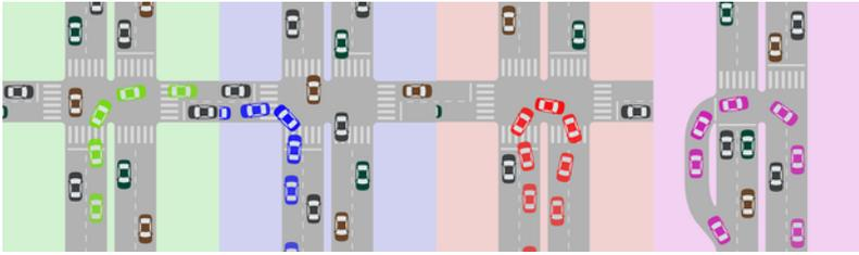
Figure 24.6. Example of a cross-traffic turn (green car), a curbside turn (blue car), a U-turn without space (red car), and a U-turn with space (pink car) for left-hand-oriented driving in India, Indonesia, South Africa, Tanzania, Australia, and the United Kingdom. *Elebeta*.
