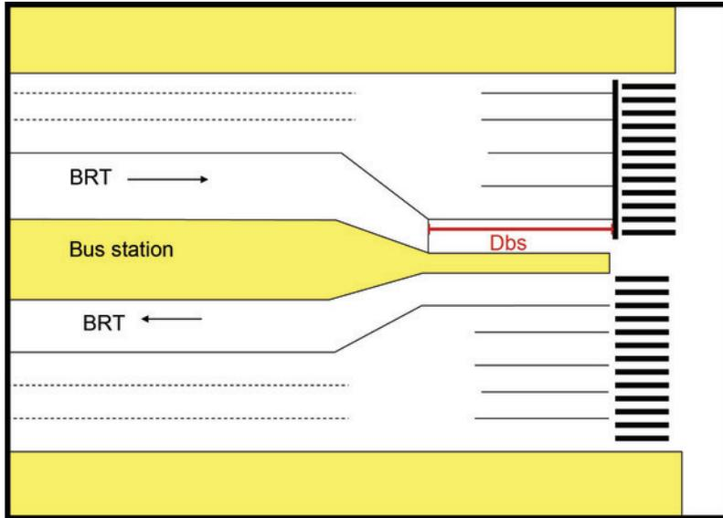
Figure 24.24. Diagram of the distance between the station and the signalized intersection ( $\text{Dist}_{\text{station-intersection}}$  shown as  $D_{bs}$ ). ITDP.
