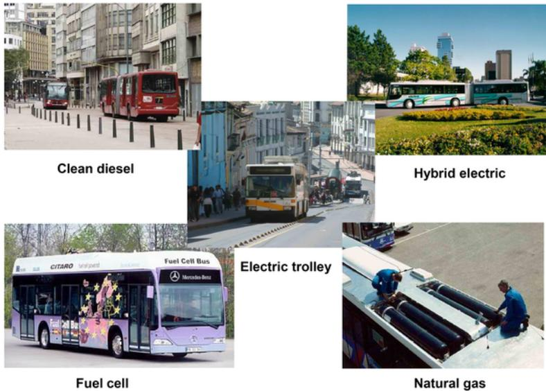
Figure 20.30. Fuel and propulsion system options. Image ITDP.
