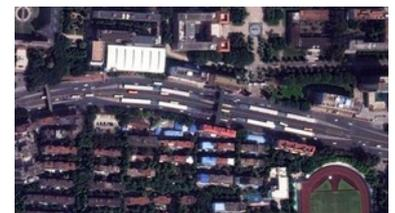
Figure 6.57. On the Guangzhou BRT, the highest capacity direct service BRT system in the world, there are stations with up to four sub-stops and twelve docking bays (two to three docking bays per sub stop) per direction. Image Bing Maps.
