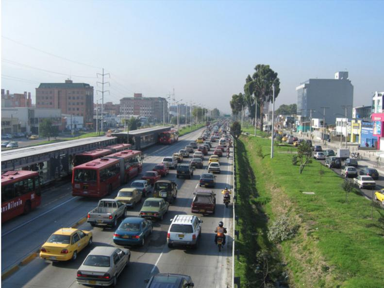
Figure 22.51. The existence of a passing lane makes the high customer capacities achieved in the Bogotá system possible. *Carlos Pardo.*
