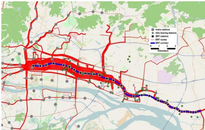
Figure 6.13. Vehicles operating on the BRT system in Guangzhou move directly from an exclusive busway to feeder routes, and thus greatly reduce the need for transfers. This image also shows bike-sharing stations implemented along the BRT corridor, and the city's metro stations. Image *ITDP*.
