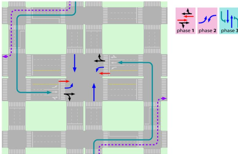
Figure 24.38. By detouring a cross-traffic turn to a curbside parallel street before reaching the intersection, a phase is eliminated in the main intersection. *Elebeta*.
