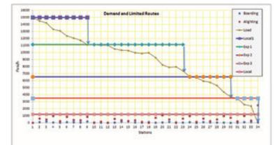
Figure 6.68. Optimal service pattern for a corridor with most demand boarding at a single terminal but alighting in even numbers at station stops along the corridor. Image Arthur Szász.
