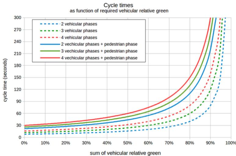
Figure 24.50. When demand requirements get too close to traffic signal capacity (overall intersection capacity) required cycles get too long very quickly. *Elebeta*.
