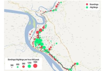
Figure 6.2. This figure shows in black the proposed BRT corridor in Yichang, China, and in green and red the estimated peak-hour boardings and alightings at all the stations on routes that are using the BRT trunk corridor. The number of existing boarding and alighting customers at each existing station will give a good preliminary indication of which stations are more important than others. ITDP.
