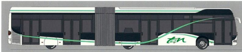
Figure 30.54. Low-floor articulated bus with four doors in Nantes, France. François Rambaud of CERTU.
