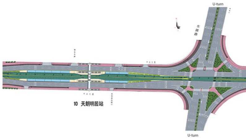
Figure 24.14. The same intersection as depicted in Figure 24.13 on a BRT corridor in Guangzhou, China. The station is located away from the intersection of the BRT corridor and Chibei Avenue. In order to turn across traffic, the two-phase intersection requires a U-turn in the perpendicular road. Before the BRT, this four-phase intersection was a major traffic-congestion point. *ITDP and GMEDRI.*
