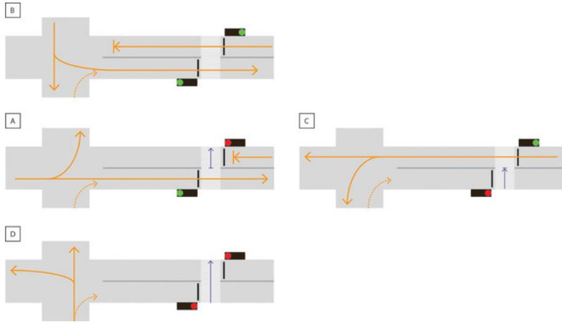
Figure 29.44. Signals can be timed to correspond to the red-and-green time at the nearest intersection to reduce the delay for mixed traffic. *ITDP*
