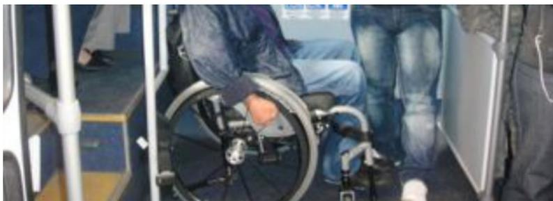
Figure 30.53. The presence of stairs between vehicle floor levels can limit the maneuvering room to get into a securement position. *Eduardo Alvarez.*
