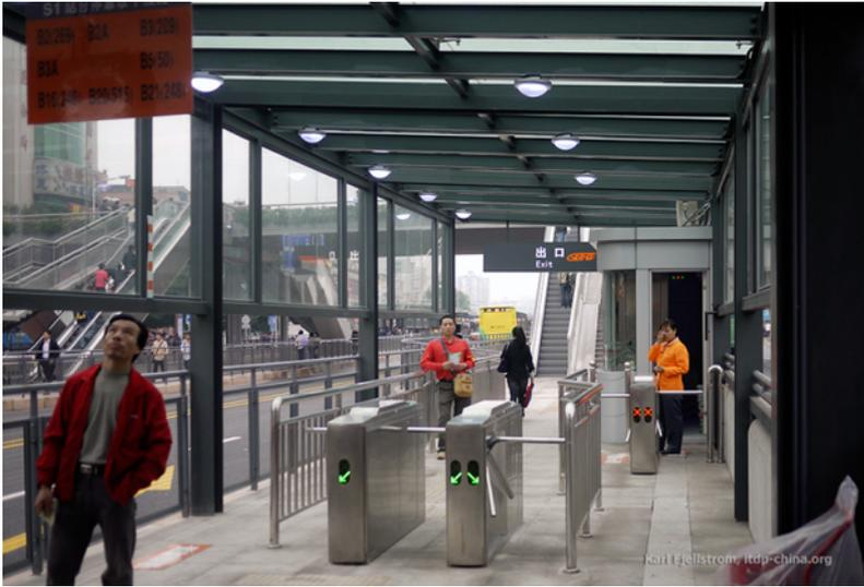
Figure 25.64. Offset turnstiles in a Guangzhou BRT station. Karl Fjellstrom
