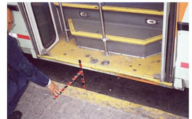
**Figure 30.62.** An ideal combination of raised vehicle stop, low first step, and proper vehicle alignment. (Each mark on the rulers equals 50 millimeters.) *Tom Rickert/AEI.*
