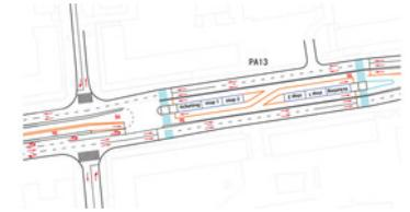
Figure 23.2. Typical conceptual layout of a BRT corridor showing dedicated lanes, intersections, stations, and station access, for a proposed BRT corridor in Ulaanbaatar, Mongolia. ITDP
