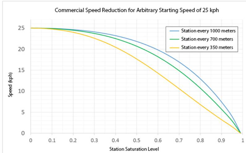
Figure 7.5. The Impact of saturation on vehicle velocity is bigger the closer the stations are to each other as each station implies more queueing delay. *Elebeta*.
