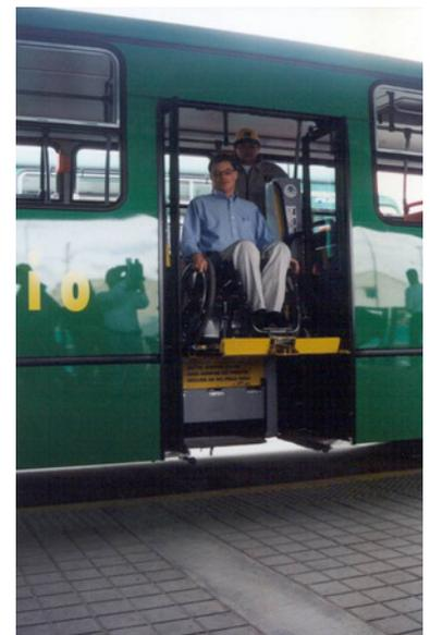
Figure 30.66. A special lift allows access for a wheelchair patron to a high-floor feeder vehicle in Bogotá. *TransMilenio SA.*
