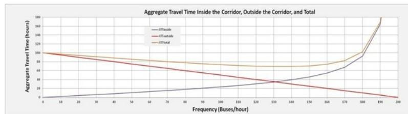
Figure 6.39. Plot of  $ATT_{i,extinside}$ ,  $ATT_{i,extoutside}$ , and  $ATT_{Total}$  for each new bus added to the corridor. The minimum aggregate travel time is reached where  $ATT_{Total}$  is the lowest, i.e., between 130 and 140 buses per hour. *Elebeta*.
