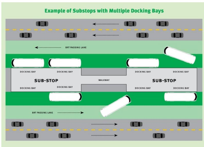
Figure 7.4. Scheme of station with two substops /ITDP
