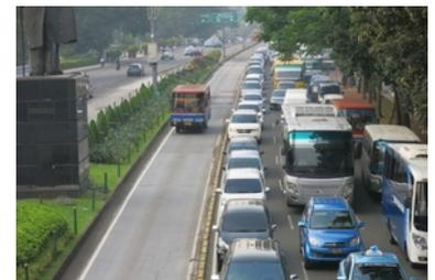
Figure 6.14. A Kopaja bus provides direct services in the TransJakarta BRT infrastructure. These buses run in mixed traffic and then enter the BRT corridor for part of their journey, but they are not officially part of the BRT system and have their own fare structure. *Aimee Gauthier.*
