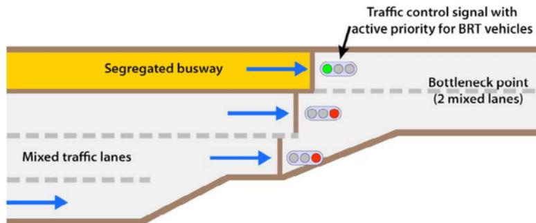
Figure 24.65. In the case of a severe bottleneck approach with traffic lights, signal priority is to be given to BRT (passive or active). ITDP
