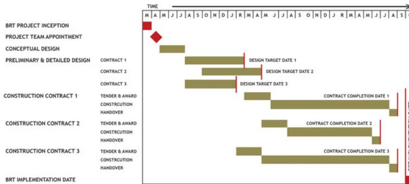
Figure 21.11. Sample timeline for a typical BRT system design and construction. HHO Africa.
