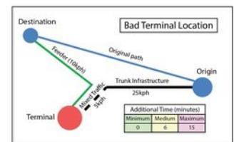
Figure 6.54. An illustration of additional route kilometers that are generated if a direct service is replaced by a trunk-and-feeder alternative where the point of transfer takes place at a facility off the BRT infrastructure. Typical terminal observations of additional customer travel times are shown in the box. Image Arthur Szász.
