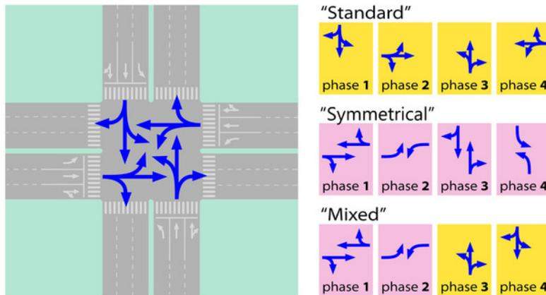
Figure 24.34. Possible movements and signal phases at a typical four-leg intersection. ITDP
