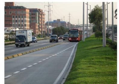
Figure 23.20. In Bogotá, the separator blocks are high enough to discourage intrusions by private vehicles but low enough to allow a BRT vehicle to leave the busway in case of emergency. *Carlosfelipe Pardo*
