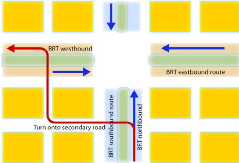
Figure 24.60. In this scenario, the BRT turning movement is made prior to the main intersection. The BRT vehicle temporarily operates on the secondary road network. ITDP.
