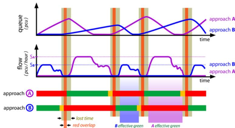
Figure 24.7. For each approach during effective green time, flow starts at saturation until the queue dissolves or the effective green time turns off. And for each approach during red time, there is queue formation, and lost time happens when neither approach has flow. *Elebeta*.
