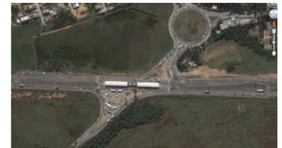
Figure 24.48. Traffic is diverted past this TransOeste station in Rio de Janeiro before it is allowed to perform U-turns away from the station. Google Earth.
