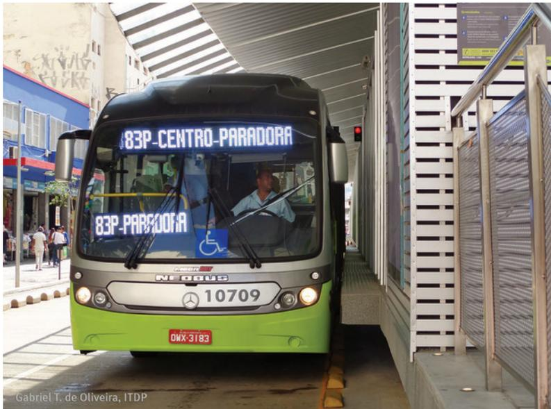
Figure 20.12. High-floor vehicles in conjunction with platform-level boarding have been the cost-effective solution for most high-quality systems in Latin America, such as the system in Belo Horizonte, Brazil. ITDP.
