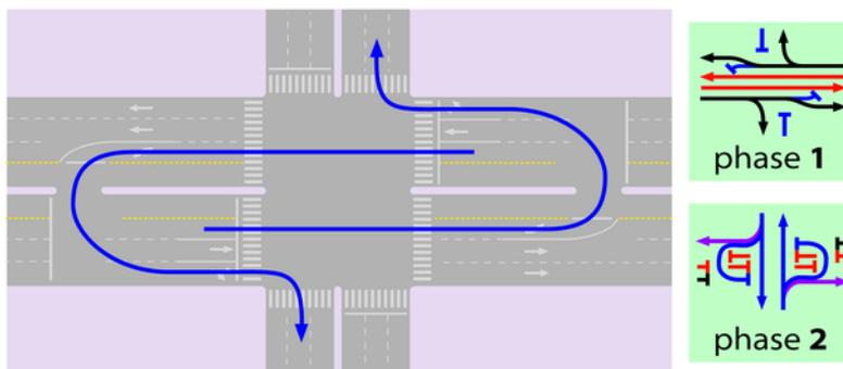
**Figure 24.43.** U-turns after crossing the intersection are an alternative to eliminate a cross-traffic-turn phase, but they require the flow to cross the intersection twice and require width for queuing downstream. *Elebeta.*
