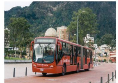
Figure 20.4. Bogotá's system uses a mix of 18-meter articulated and 24-meter bi-articulated vehicles. TransMilenio SA.
