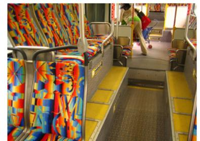
Figure 30.50. Irregular floor plans reduce internal accessibility. *Tom Rickert/AEI.*
