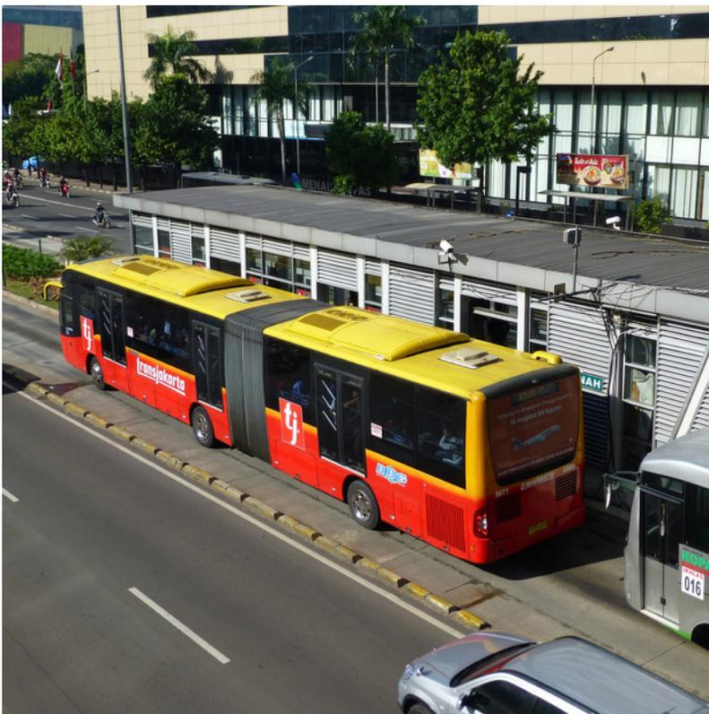
Figure 22.12. TransJakarta utilizes buses with doorways on both sides of the vehicle in order to service both median and curbside stations. *ITDP.*
