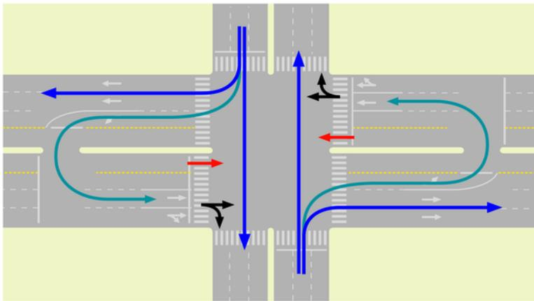
**Figure 24.42.** Making a U-turn after entering, by means of a curbside turn, the opposite way of the desired direction is another way to perform a cross-traffic turn without need of an exclusive phase. This alternative requires a queuing area and uses two approaches to the intersection as well. *Elebeta.*
