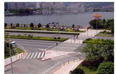
Figure 29.25. A median in the center of the road keeps drivers from swinging wide during a turn in Shenzhen, China. *Karl Fjellstrom, Far East BRT*
