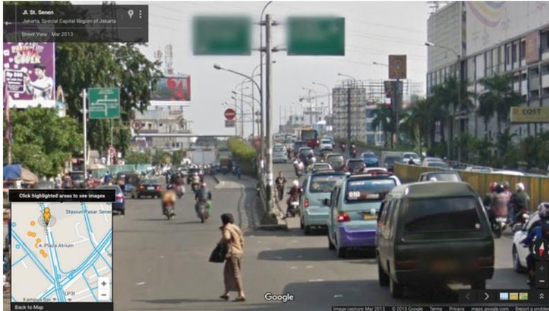
Figure 24.83. In Senen Street, Transjakarta interlaces with mixed traffic to avoid the flyover and reach the station near the intersection. The restart of the bus lane is on the ground level, close to the flyover. The flyover has two lanes and only two more are available to reach the intersection below it. The covered pedestrian flyover seen at the left is a link between the inside area of stations in BRT Corridor 2 and Corridor 6 as the user cannot leave the system's "paid areas." Google Maps.
