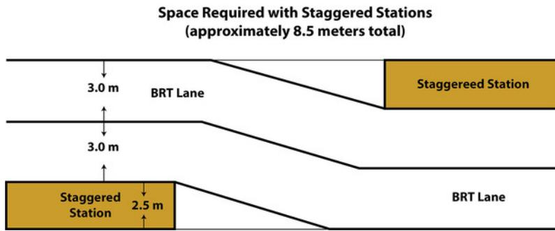
Figure 22.64. Relative space requirements for roadway configurations with staggered stations. *HHO Africa*.
