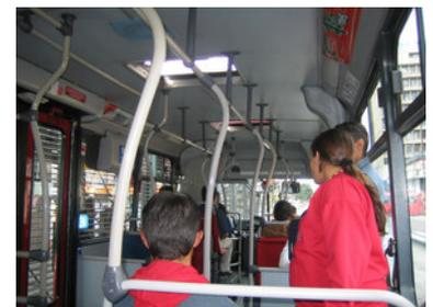
Figure 30.55. Vertical stanchions and grab bars are provided on TransMilenio to assist customers; however, better color contrast is needed. TransMilenio.
