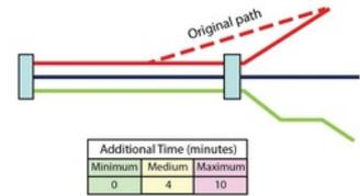
Figure 6.53. An illustration of why additional route kilometers would be added to a route if it were converted to a trunk-and-feeder route and the point where the new transfer takes place (a new transfer facility) is beyond the point where the original route diverged from the trunk route. Typical terminal observations of additional customer travel times are shown in the box. Image Arthur Szász.
