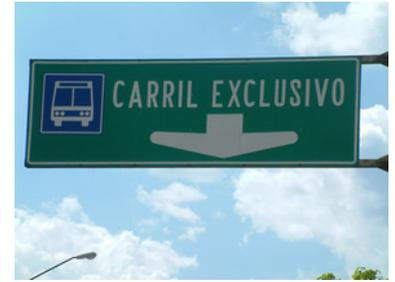
Figure 23.26. Signage is a basic mechanism to designate an exclusive busway. This example is from León, Mexico. Karl Fjellstrom
