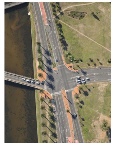
Figure 24.59. Pre-signals for buses, holding normal vehicles in Cape Town, South Africa, work like a queue jump to a straight movement in a mixed-traffic section. *Bruce Sutherland.*
