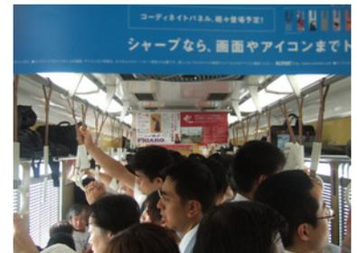
Figure 11.21. Visual clutter from hanging advertisements in Japanese rail systems can hamper the customer’s ability see other information, such as system maps, as well as reduce outside visibility. Photo courtesy of Lloyd Wright.
