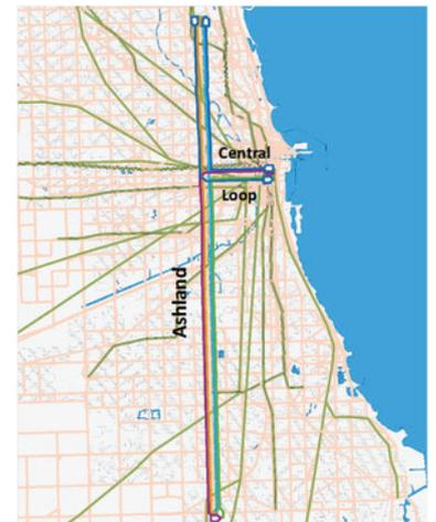
Figure 6.72. For the Ashland and Central Loop BRT projects in Chicago, original typical grid-pattern bus services will not optimally serve the demand when converted to BRT. Image Pedro Szász.
