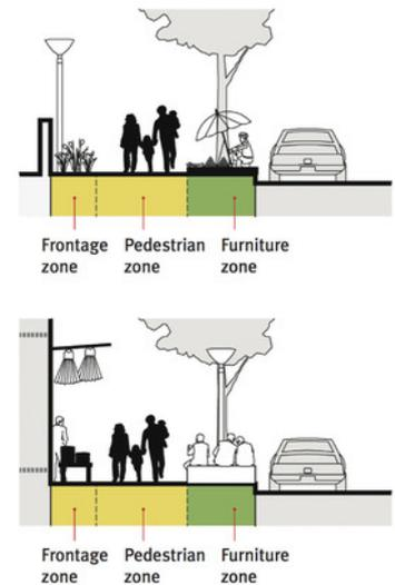
**Figure 29.16.** Sidewalks should include a frontage zone to buffer adjacent land uses and a furniture zone to accommodate underground utilities, trees, and furniture in order to ensure that the pedestrian zone remains free of encroachments or obstacles. *Diagram courtesy of ITDP’s Better Streets, Better Cities (2011)*
