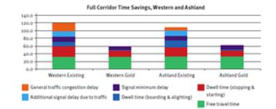
Figure 5.9. Causes of bus delay for two corridors in Chicago and how Gold Standard BRT can help reduce this delay. ITDP.
