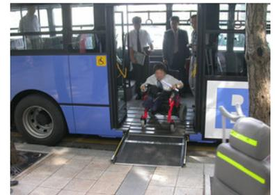
Figure 30.65. A manually operated ramp extended from the vehicle provides access for wheelchair users. *City of Seoul.*
