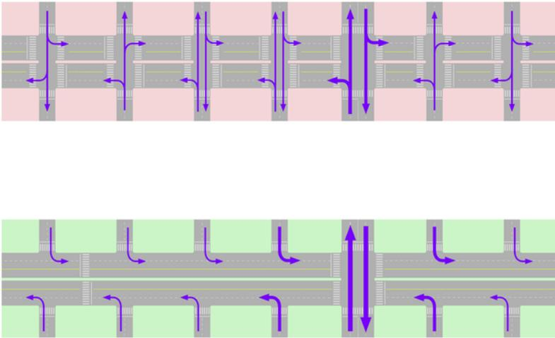
Figure 24.32. Closing intersections reduces accessibility, and may lead to harder to handle intersections. With no stations, BRT vehicles can benefit from signal coordination. *Elebeta.*
