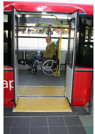
Figure 30.49. The wheelchair securement area is reached quickly on most high-floor vehicles. *City of Cape Town.*
