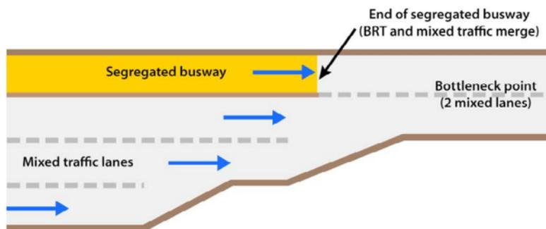
Figure 24.64. In the case of a severe bottleneck point, it may be best to terminate the exclusivity of the busway prior to reaching the bottleneck. ITDP
