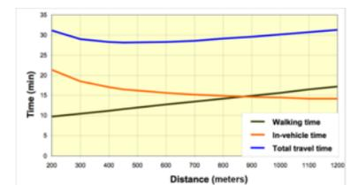
Figure 6.59. Optimizing total travel time as a function of station separation, this graph illustrates the trade-off faced by customers for increasing distances between station stops. As station stop distances increase, in-vehicle time falls as BRT vehicle speeds increase, but walking times also increase. Total travel time in a typical urbanized corridor tends to become minimal with stop distances around 450 meters. Image Arthur Szász.
