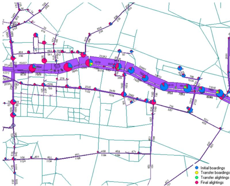
Figure 4.18. Projected morning peak customer flows along the Guangzhou BRT, with BRT customer volumes marked for each link along the corridor. *ITDP*.
