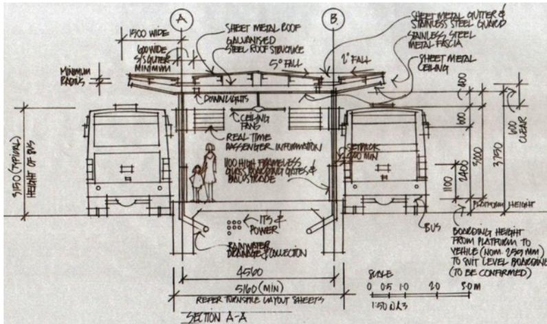
Figure 25.55. Proposed station dimensions for a BRT conceptual design by ITDP in Malaysia. The BRT door height is 1.1 meters. For fully enclosed stations an extra height of at least 0.5 meters is recommended. ITDP and created by Derek Truster.
