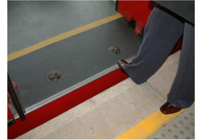
Figure 7.21. Reducing the board gap, as seen here in Bogotá, Colombia, allows customers to safety board and alight faster, increasing system capacity. Lloyd Wright.
