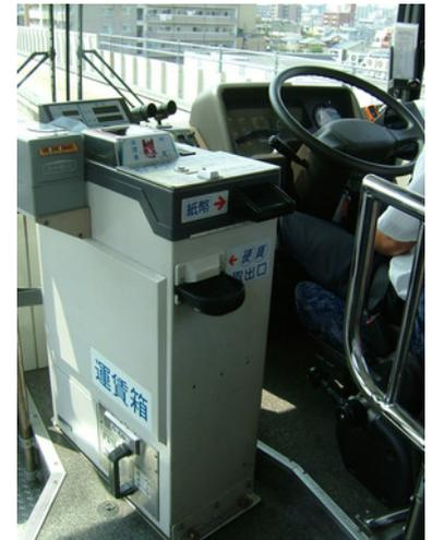
Figure 18.3. All-purpose bus fare collection machine in Nagoya, Japan. Karl Fjellstrom.
