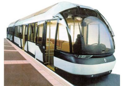
Figure 20.41. Despite giving a distinctly light-rail appearance, the Cavis vehicle is actually a bus. US TCRP media library.
