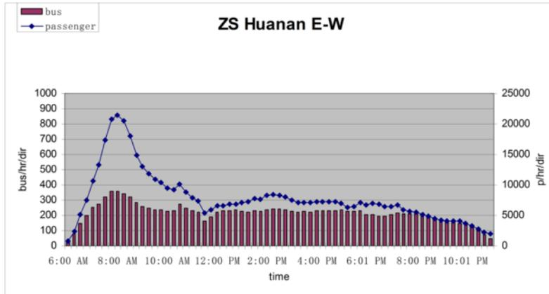
Figure 4.11. Sample graph of bus and customer counts in a single direction at a high demand location on the then-planned Guangzhou BRT in peak and off-peak periods, with customer flows exceeding 20,000 customers and 350 buses per hour in an east-west direction. *ITDP*.
