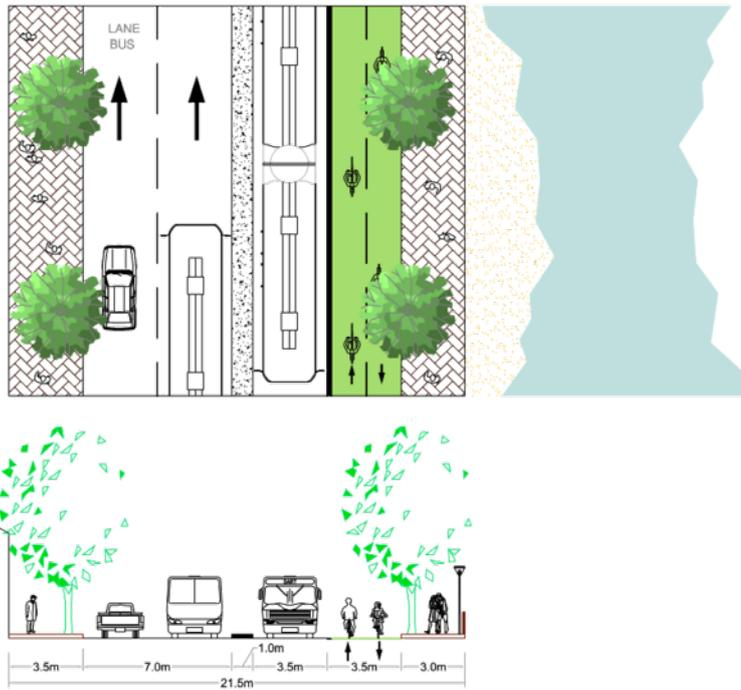
Figure 22.15. Plan and section view of Stretch 1 at a width of 21.5 meters. Logit.
