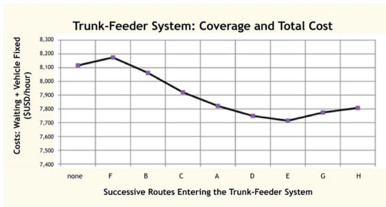
Figure 6.52. Likely cost curve for feeder routes of various travel times but where in general feeder route travel times are short relative to total travel time. *Pedro Szász.*
