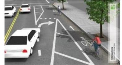
Figure 31.19. A "mixing" zone at an intersection. Typically the cyclist swings to the left of the right-turning driver. *NACTO.*
