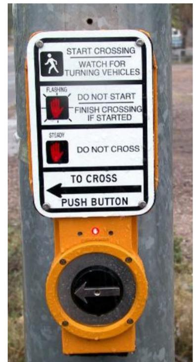
Figure 30.18. A vibro-tactile pushbutton for requesting a crossing phase. *Janet Barlow.*
