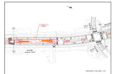
Figure 21.8. ITDP China's preliminary design drawing for a BRT station, intersection, and roadway in Yichang, China. *ITDP and the Guangzhou Municipal Engineering Design & Research Institute.*
