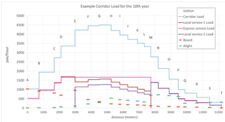
Figure 7.8. Example corridor morning peak loads for the tenth year, boarding and alighting per station. Image Ele-beta.
