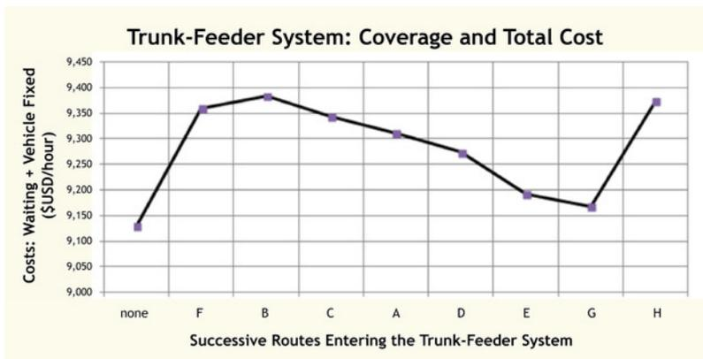
Figure 6.51. Likely cost curve if there are feeder routes of varying length but in general the time spent on the feeder route is long relative to the time spent on the trunk route. Graph *Pedro Szász*.
