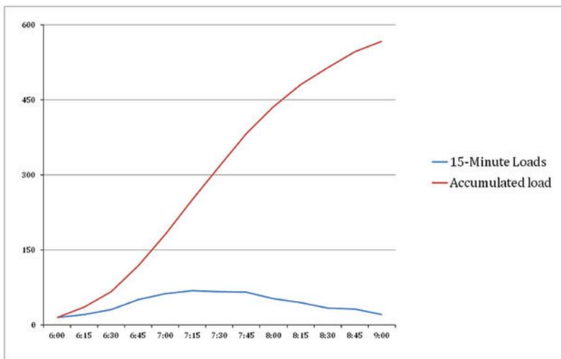
Figure 6.25. The graph shows 15-minute loads (blue) versus overall accumulated loads (red). Peak 15-minute period occurs where blue curve hits its max, or 7:00–7:15 a.m. *Arthur Szász.*
