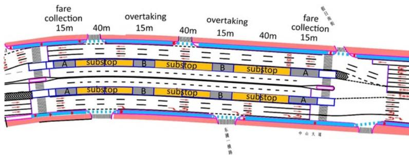
Figure 25.14. Dongpu BRT station in Guangzhou in plan view shows more clearly the parts of the station, which consists of 3 sub-stops in each direction, with a total length of 180m. Each sub-stop consists of 2 docking bays for 18m BRT buses, or 3 sub-stops for 12m BRT buses. A = fare collection and B = passing area. The platform is 5m wide. *ITDP China and GMEDRI.*
