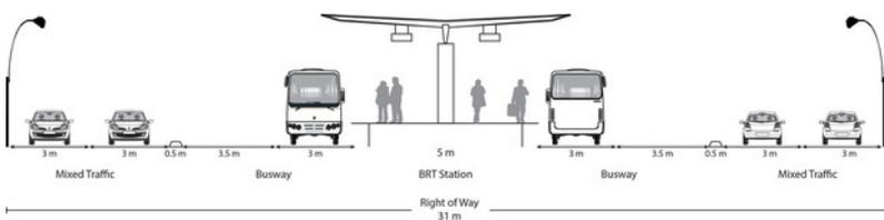
Figure 22.2. A conceptual design of a BRT corridor. ITDP.
