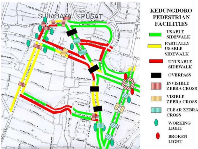
Figure 29.58. Results of street audit for Surabaya, Indonesia, with the quality of the pedestrian environment color-coded according to usability: green, usable; yellow, partially usable; and red, unusable. GIZ and ITDP
