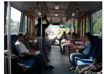
Figure 20.16. Side-facing seating, as shown in this example from Jakarta, Indonesia, will tend to maximize space for standing customers, and thus such a configuration will maximize overall customer capacity per vehicle. Karl Otto, courtesy of GLZ.
