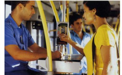
Figure 7.28. In Brazil, a "reservoir" space is provided within the vehicle where customers line up to verify their fare. With the use of this reservoir, the vehicle is able to proceed even before all customers have verified their fare. *The Municipality of Goiânia.*
