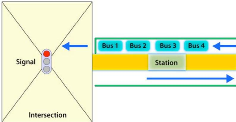
Figure 24.25. For the direction of the BRT system that stops at the station before the intersection, there is a risk that vehicles will be delayed due to the signal phase. *ITDP*.
