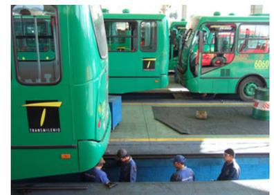
Figure 26.2. At the Usme depot in Bogotá, the green feeder vehicles are maintained at the same facility as the red trunk vehicles. Lloyd Wright.
