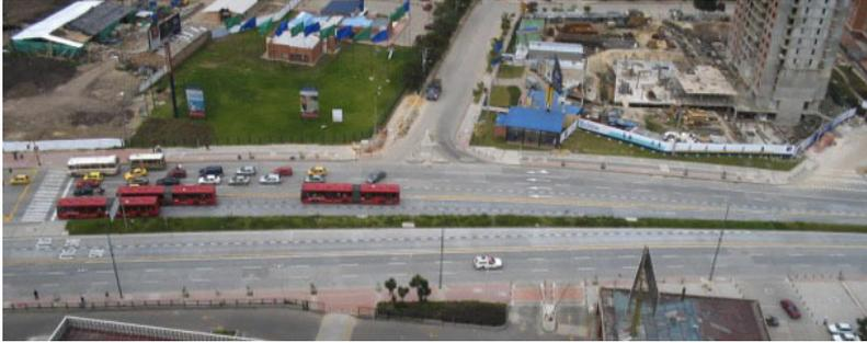
Figure 24.16. Single to double lanes just before the intersection in Bogotá to ensure proper capacity. Oscar Edmundo Diaz, GSD+.
