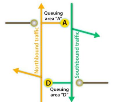
Figure 24.63. Vehicle movements for signal phase 2 in a cross converted into roundabout. ITDP.
