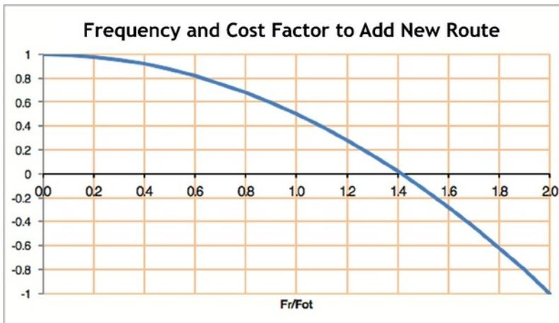
Figure 6.60. The cost factor of splitting a route into a local route and a new limited-stop route when the relation of frequency to optimal frequency ( $\frac{Fr}{Fot}$ ) is considered: When the frequency rises above 31 ( $\frac{31}{22=1.4}$ ) the benefit from reduced service irregularity is greater than the time lost waiting for a lower frequency service. Arthur Szász.
