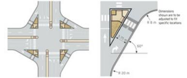
Figure 29.26. A pedestrian island, in conjunction with a tightened turning radius (right), can do much to benefit pedestrian safety (left). *Emirate of Abu Dhabi*
