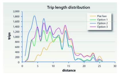
Figure 15.4. Analysis of the impact of different fare structures on TransJakarta's Phase II ridership. ITDP.
