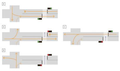
Figure 29.44. Signals can be timed to correspond to the red-and-green time at the nearest intersection to reduce the delay for mixed traffic. *ITDP*
