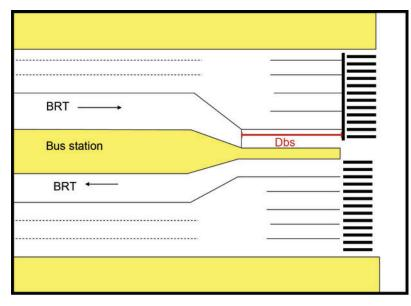
$\text{Dist}_{\text{station-intersection}}[\text{in meters}] \geq 2.5*90 = 225$
