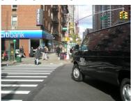
Figure 29.29. Vehicle phase of a leading pedestrian interval in New York City in which vehicles are given a green light only after pedestrians are allowed to begin crossing *Michael King*
