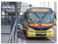
Figure 7.24. The presence of the boarding bridge means that the driver does not need to be as precise docking at the platform. In turn, this can significantly reduce the time lost at stations. Image *Lloyd Wright*.
