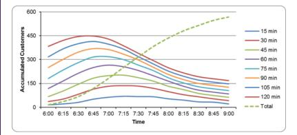
**Figure 6.26.** Accumulated demands for varying cycle times, using the same data as in Tables 6.13 – 6.15. *Arthur Szász*.
