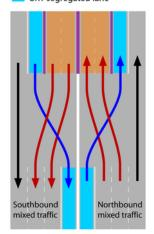
Figure 24.82. Schematic of Delhi roadway in which BRT vehicles must cross mixed traffic that is attempting to access a flyover. Image *Elebeta*.
