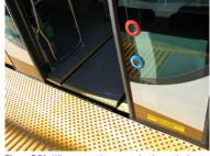
Figure 7.31. When operating properly, the optical guidance system employed in Las Vegas, Nevada, USA, can align the vehicle within a few centimeters of the platform. *NBRTI*.
