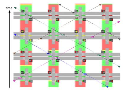
Figure 24.8. Traffic light coordination can provide green waves to several routes by synchronizing the opening of green phases with the flow speed. Image *Elebeta*.
