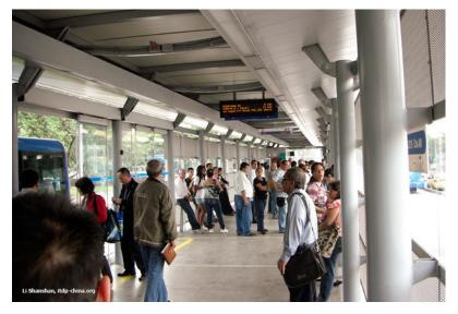
Figure 25.79. BRT station interior in Cali. The doors are offset so that passengers waiting for buses in one direction do not conflict with the passengers waiting for buses in the other direction. Shanshan Li, ITDP
