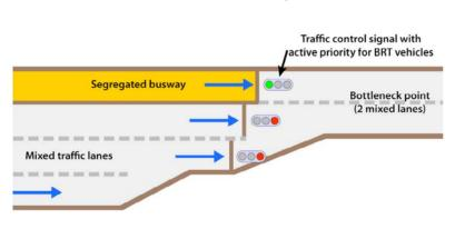
Figure 24.65. In the case of a severe bottleneck approach with traffic lights, signal priority is to be given to BRT (passive or active). *ITDP*
