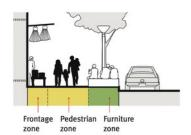
Figure 29.16. Sidewalks should include a frontage zone to buffer adjacent land uses and a furniture zone to accommodate underground utilities, trees, and furniture in order to ensure that the pedestrian zone remains free of encroachments or obstacles. *Diagram courtesy of ITDP's Better Streets, Better Cities (2011)*
