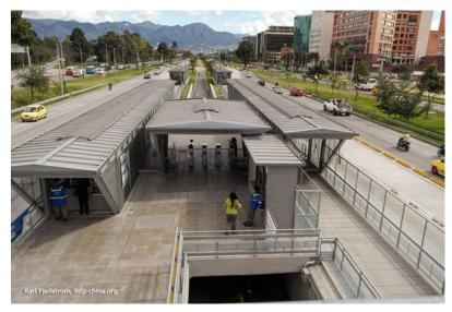
Figure 25.63. Straight row of turnstiles in a Bogotá BRT station with a segregated bike lane passing under the station. Karl Fjellstrom
