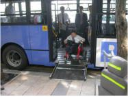
Figure 30.65. A manually operated ramp extended from the vehicle provides access for wheelchair users. *City of Seoul.*
