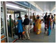
Figure 7.20. With well-designed infrastructure and adequate driver training, such as in Ahmedabad, India,BRT systems can reduce the boarding gap to under 10 centimeters Shreya Gadepalli
