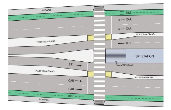
Figure 29.53. Pedestrian islands should be constructed between the busway and mixed traffic lanes. ITDP
