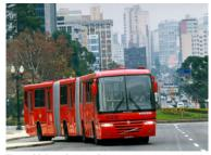
Figure 20.3. In Curitiba, 24-meter bi-articulated vehicles are utilized on trunk corridors. Volvo Bus Corporation.
