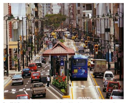
Figure 22.41. Through the denser city center area, the Guayaquil Metrovía system utilizes a split-route configuration, with each direction of travel being provided on parallel streets. *Carlos González*.
