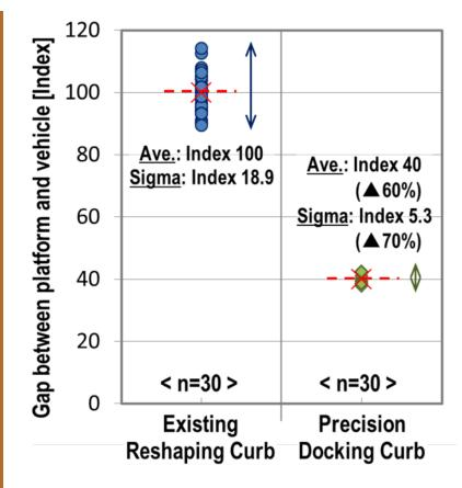
Figure 25.97. The gap improvement from using the precision docking curb method. Bridgestone
