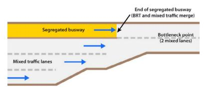
Figure 24.64. In the case of a severe bottleneck point, it may be best to terminate the exclusivity of the busway prior to reaching the bottleneck. *ITDP*
