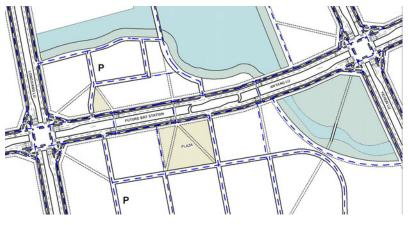
Figure 31.6. A design for a bicycle network in tandem with a BRT network in Harbin, China. Bicycle routes are denoted by dotted blue lines. *NelsonWygaard*.
