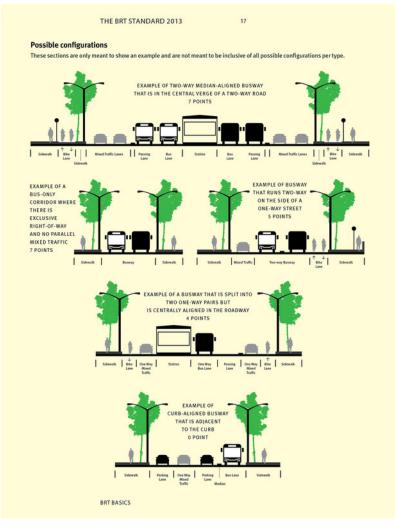
Figure 22.8. Examples of different BRT roadway configurations from The BRT Standard. ITDP.
