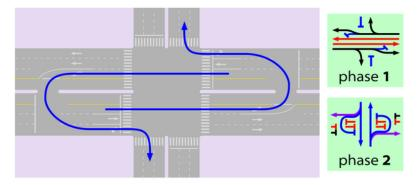
Figure 24.43. U-turns after crossing the intersection are an alternative to eliminate a cross-traffic-turn phase, but they require the flow to cross the intersection twice and require width for queueing downstream. *Elebeta*.
