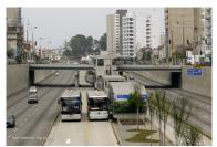
Figure 25.43. Offset central platforms in Lima with passing lanes and sub-stops. *Karl Fjellstrom*.
