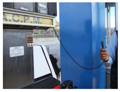
Figure 26.4. Upon entering the refueling area, a digital monitoring device records the pertinent vehicle details (i.e., fuel level, odometer, etc.). *Lloyd Wright*.
