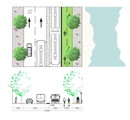
Figure 22.15. Plan and section view of Stretch 1 at a width of 21.5 meters. Logit.
