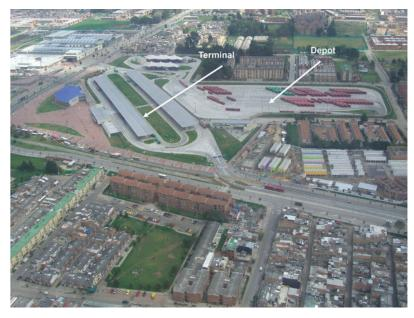
Figure 26.1. In Bogotá, most depots are located next to the terminal areas in order to improve operational efficiency. Oscar Diaz and Por el País que Queremos (PPQ).
