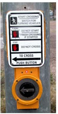
Figure 30.18. A vibro-tactile pushbutton for requesting a crossing phase. Janet Barlow.
