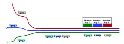
Figure 7.6. Convoying systems order vehicles when entering the corridor, so they ride as "train" and the docking position for every route at the station is fixed, preventing users from running up and down the platform. Pedro Szász.
