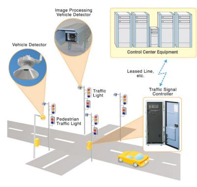
Figure 19.9. Signal control system. Sumitomo Electric.
