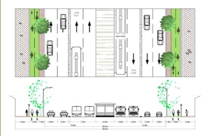
Figure 22.16. Plan and section view of Stretch 5 at a width of 49 meters. Logit.
