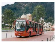
Figure 20.4. Bogotá's system uses a mix of 18-meter articulated and 24-meter bi-articulated vehicles. *TransMilenio SA*.
