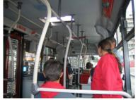
Figure 30.55. Vertical stanchions and grab bars are provided on TransMilenio to assist customers; however, better color contrast is needed. *TransMilenio*.
