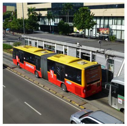
Figure 22.12. Translakarta utilizes buses with doorways on both sides of the vehicle in order to service both median and curbside stations. *ITDP*.
