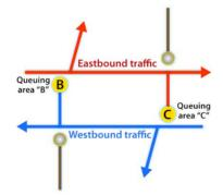
Figure 24.62. Vehicle movements for signal phase 1 in a cross converted into a roundabout. *ITDP*.
