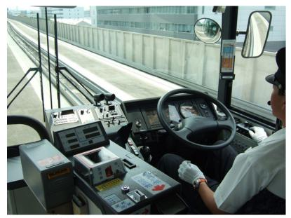
Figure 22.29. The guideway allows for hands-free driving on the Nagoya-Yutorito Line. Lloyd Wright.
