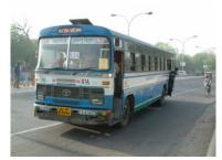
Figure 20.29. All public-transport vehicles in Delhi, including the oldest vehicles, faced a mandatory conversion to CNG fuel in order to overcome difficulties with adulterated fuels. *Lloyd Wright*
