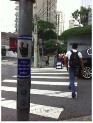
Figure 24.9. As an example of actuation, pedestrians may "call the controller for a service" by pressing a button, as in this crossing in São Paulo. Jonas Malaco.
