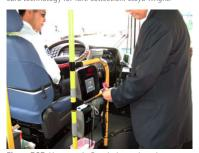
Figure 7.27. However, in Seoul, the on-board nature of the fare verification means that dwell times are negatively affected. A single customer searching through personal effects for his or her smart card can create a significant delay. *Lloyd Wright*.
