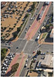
Figure 24.29. Cape Town, South Africa's standard four-phase intersection with a cross-traffic-turn waiting area using the narrowed width of the opposite way. *Bruce Sutherland*.
