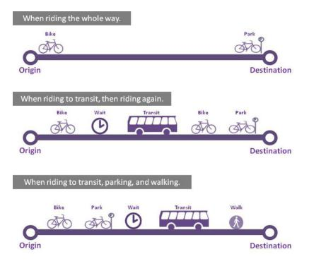
Figure 31.1. Comparison of various trip chains involving the bicycle, public transport, and walking. TransLink
