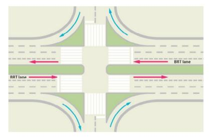
Figure 24.70. The introduction of a pedestrian island between the curbside-turn lane and the crossing can significantly help pedestrians safely cross within the standard two-phase traffic signal. *ITDP*.
