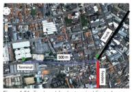
Figure 6.56. Trunk-and-feeder terminal Santo Amaro in São Paulo is poorly located and accesses are poorly designed, causing additional travel times. Image *Arthur Szász*.
