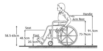
Figure 20.23. Wheelchair dimensions and the anthropometric measurements indicated in the preceding diagrams should be considered in sizing the backrest. *ITDP*
