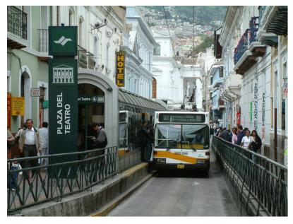
Figure 22.18. Insertion of bus lane and station in a narrow space in Quito. Andre Frieslaar.
