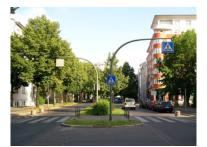
Figure 29.42. Example in Berlin of a pedestrian cross walk with vertical elements indicating to drivers the location of the crosswalk. *Michael King*
