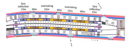
Figure 25.14. Dongpu BRT station in Guangzhou in plan view shows more clearly the parts of the station, which consists of 3 sub-stops in each direction, with a total length of 180m. Each sub-stop consists of 2 docking bays for 18m BRT buses, or 3 sub-stops for 12m BRT buses. A = fare collection and B = passing area. The platform is 5m wide. *ITDP China and GMEDRI*.
