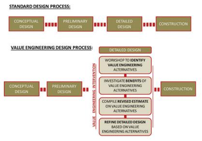
Figure 21.13. Standard- and value-design engineering process flow diagrams. HHO Africa.
