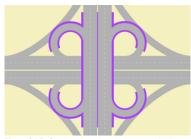
Figure 24.3. Separated-grade solutions can eliminate intersections. *Elebeta*.
