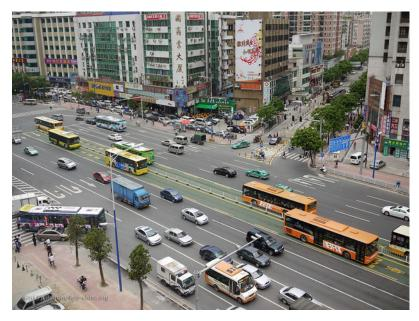
Figure 24.46. This intersection near Dongpu BRT Station in Guangzhou was previously a major traffic black spot-a location where traffic accidents often occurred—but now it works very smoothly for all modes, with a two-phase signal combined with U-turns and pedestrian crossings. *Karl Fjellstrom, ITDP*.
