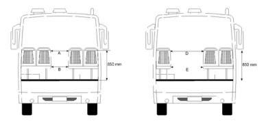
Figure 20.19. The aisle located between the doors in all types of vehicles must not have double seats on both sides. ITDP
