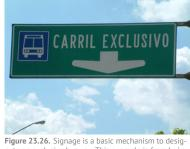
**Figure 23.26.** Signage is a basic mechanism to designate an exclusive busway. This example is from León, Mexico. *Karl Fjellstrom*
