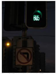
Figure 24.17. Active signal priority for BRT and restricted turning movements for vehicles in mixed traffic can do much to improve public transport travel times. *Lloyd Wright*.
