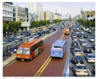
Figure 24.23. A mid-block station location in Seoul allows greater right-of-way width for the station area. *City of Seoul*.
