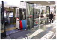
Figure 30.33. Sliding doors are a feature of many BRT systems. *ITDP*
