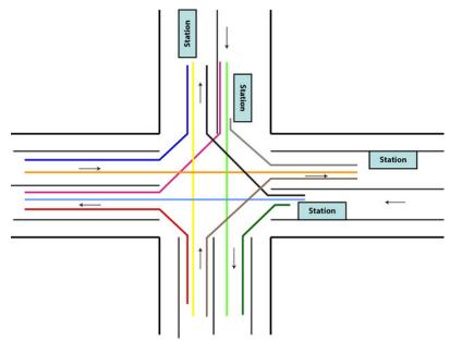
Figure 22.61. An alternative means of connecting split and side-aligned stations is to provide a full set of route permutations. *HHO Africa*.
