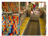
Figure 30.50. Irregular floor plans reduce internal accessibility. *Tom Rickert/AEI*.
