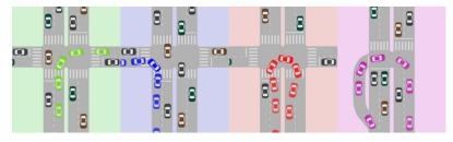
Figure 24.6. Example of a cross-traffic turn (green car), a curbside turn (blue car), a U-turn without space (red car), and a U-turn with space (pink car) for left-hand-oriented driving in India, Indonesia, South Africa, Tanzania, Australia, and the United Kingdom. *Elebeta*.
