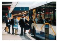
Figure 20.11. Low-floor vehicles without platformlevel entry and pre-board fare verification can result in longer dwell times and not actually provide access to the physically disabled, as shown in this images from Brisbane, Australia Queensland Transport.
