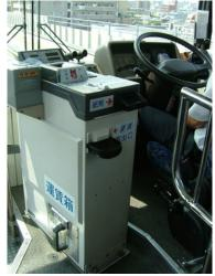
Figure 18.3. All-purpose bus fare collection machine in Nagoya, Japan. Karl Fjellstrom.
