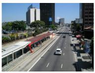
Figure 29.47. In São Paulo, this mid-block station is served by a pedestrian overpass, but does not have physical separation to keep customers from crossing travel lanes to access buses. *Michael King*
