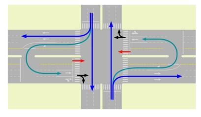
Figure 24.42. Making a U-turn after entering, by means of a curbside turn, the opposite way of the desired direction is another way to perform a cross-traffic turn without need of an exclusive phase. This alternative requires a queueing area and uses two approaches to the intersection as well. *Elebeta*.
