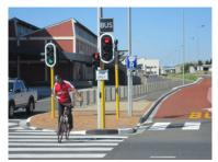
Figure 23.18. In Cape Town, South Africa, the separator between the busway and the mixed-traffic vehicles acts as a two-way bike lane and an island for pedestrians. *ITDP*
