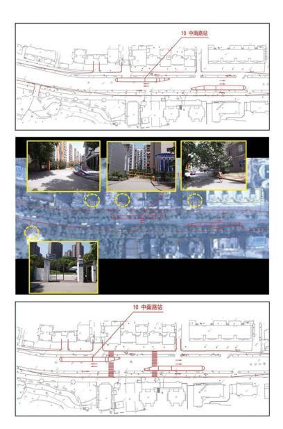
Figure 29.55. This series of images from Yichang, China, shows how a BRT station location is slightly adjusted to better serve the surrounding pedestrian network. The top image shows the initial layout. The second image locates adjacent streets and crossing opportunities. In the last image, the station has been moved to the left and crosswalks added. *ITDP*
