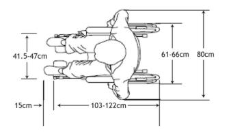
Figure 20.22. Wheelchair dimensions and the anthropometric measurements indicated in the preceding diagrams should be considered in sizing the backrest. *ITDP*
