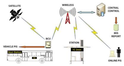
Figure 19.1. The automatic vehicle location system. Prodigy Electronics.
