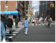
Figure 29.28. Pedestrian phase of a leading pedestrian interval in New York City. Pedestrians are permitted to begin crossing the intersection before vehicles get a green light. *Michael King*
