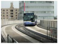
Figure 22.27. Nagoya, Japan's elevated BRT line uti lizes a mechanical guidance system to reduce the required roadway width. *Lloyd Wright*.
