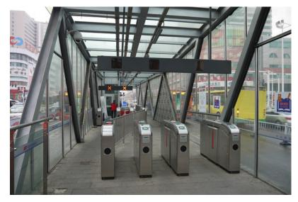
Figure 18.6. Urumqi, China, streamlines customer flow by offsetting the gates and making them unidirectional. Image Karl Fjellstrom.
