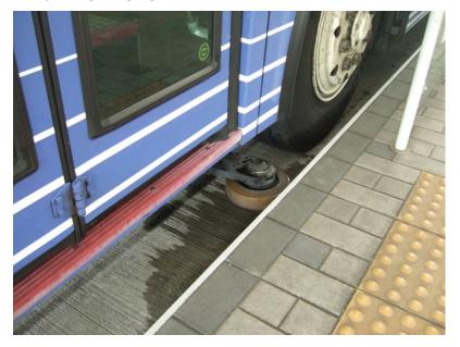
Figure 22.26. Nagoya, Japan's elevated BRT line utilizes a mechanical guidance system to reduce the required roadway width. *Lloyd Wright*.
