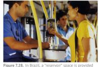
Figure 7.28. In Brazil, a "reservoir" space is provided within the vehicle where customers line up to verify their fare. With the use of this reservoir, the vehicle is able to proceed even before all customers have verified their fare. The Municipality of Goidnia.
