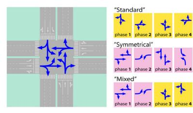
Figure 24.34. Possible movements and signal phases at a typical four-leg intersection. ITDP.
