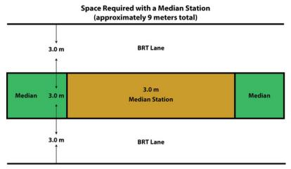
Figure 22.63. Relative space requirements for roadway configurations with median stations. HHO Africa.
