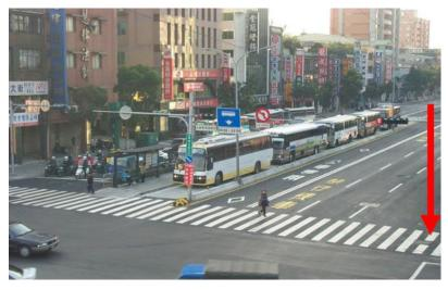
Figure 24.27. For the direction of the BRT system that stops after the intersection, there is a risk that vehicles create a backup into the intersection and block traffic. *ITDP*
