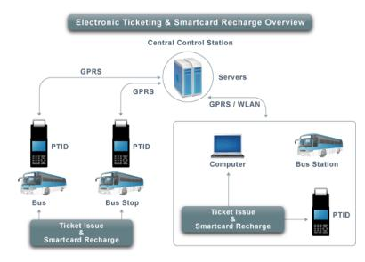
Figure 19.4. Electronic Ticketing and Smart Card Recharge Overview. Prodigy Electronics.
