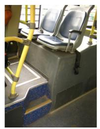
Figure 30.51. Irregular seating plans reduce internal accessibility. *Tom Rickert/AEI*.
