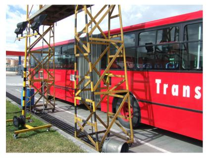
Figure 26.7. Scaffolding permits the tops of the vehicles to be washed *Lloyd Wright*.
