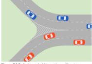
Figure 24.2. A channeled Y junction without conflicts does not have the basic element that defines an intersection. *Elebeta*.
