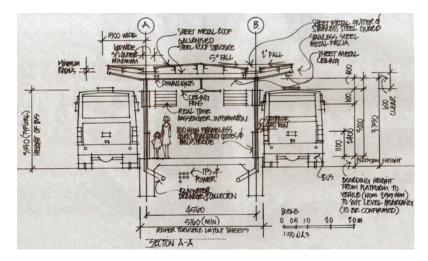
Figure 25.55. Proposed station dimensions for a BRT conceptual design by ITDP in Malaysia. The BRT door height is 1.1 meters. For fully enclosed stations an extra height of at least 0.5 meters is recommended. *ITDP and created by Derek Trusler.*
