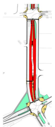
Figure 22.53. An intermediate transfer station on Cape Town's MyCITI system, with a closed environment between the trunk platform on the left and the feeder platform on the right. *Planning Partners*.
