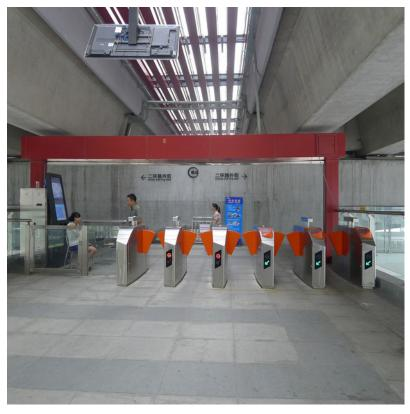
Figure 18.5. The BRT system in Chengdu, China, utilizes wing gates to control access to the system. Karl Fjellstrom.
