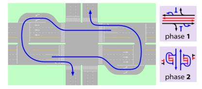
Figure 24.44. Waiting area for a U-turn can be placed closer to the curb, instead of close to the median. Elebeta.
