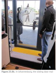
Figure 25.86. In Johannesburg, the sliding door malfunctioned and did not open as the bus pulled up, leaving the passenger stranded between the bus and station. The station attendant quickly came to manually open the doors with a remote control. *ITDP*
