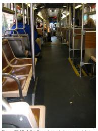
Figure 30.48. A flat floor of a high-floor articulated bus in San Francisco. *Tom Rickert/AEI*.
