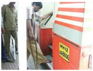
Figure 30.61. A low first step makes boarding easier. The man is stepping into the vehicle without lifting his body or bending his knee. Once within the stairwell, he is then better able to use his upper body strength to mount the remaining stairs. *TRL Ltd.*
