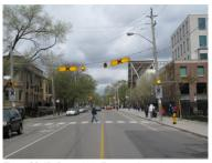
Figure 29.43. Example in Toronto of a pedestrian crosswalk with vertical elements indicating to drivers the location of the crosswalk. *Michael King*
