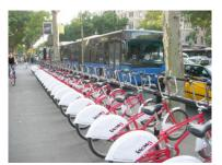
Figure 31.53. Barcelona's bike-share system features sturdy bicycles with internal gearing, fenders, chain guards, and front baskets. *Nelson*/Wyaaard.
