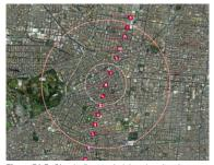
Figure 31.3. Bicycle (larger circle) and pedestrian (smaller circle) catchment areas overlaid on stations along the Insurgentes BRT line in Mexico City. *Google Earth.*
