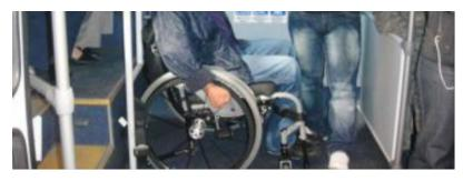
Figure 30.53. The presence of stairs between vehicle floor levels can limit the maneuvering room to get into a securement position. Eduardo Alvarez.
