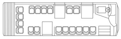
Figure 20.16. Side-facing seating, as shown in this example from Jakarta, Indonesia, will tend to maximize space for standing customers, and thus such a configuration will maximize overall customer capacity per vehicle. *Karl Otta, courtesy of GIZ*.
