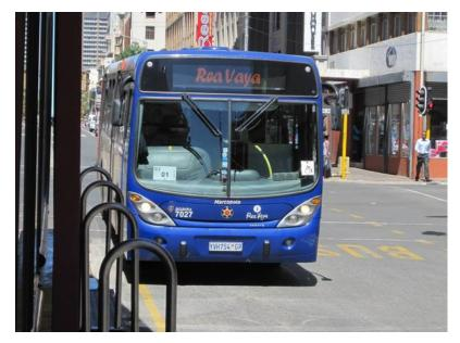
Figure 25.90. In Johannesburg, bus drivers line up the yellow line on the dashboard to the yellow line on the pavement to dock closely to the station. *ITDP*
