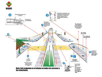
Figure 30.9. Pedestrian-access features are depicted in this diagram of approaches to a typical BRT station on Avenue Simón Bolívar in Pereira, Colombia. *Pereira Megabús*.
