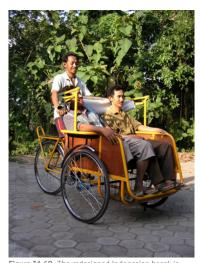
Figure 31.60. The redesigned Indonesian becak is lighter and more stable than traditional models. *ITDP*.
