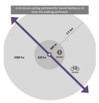
**Figure 31.2.** Cycling catchment area compared to walking catchment area. *TransLink*
