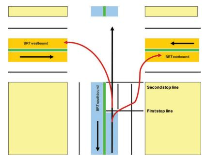
Figure 24.58. While mixed-traffic vehicles are held for an extra ten seconds at the first traffic-signal stop, BRT vehicles are given a queue-jumping head start. Technically this counts as eight phases. TCRP
