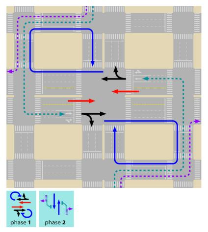
Figure 24.39. Three curbside turns after crossing the intersection is a simple alternative to eliminating cross-traffic turns; despite crossing the intersection twice, it does not create much conflict with existing flows. *Elebeta*.
