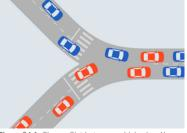
Figure 24.1. The conflict between vehicles in a Y junction indicates that this is an intersection. *Elebeta*.
