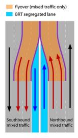
Figure 24.84. Alternative design for a flyover that allows BRT vehicles to proceed without conflicts to the area below the flyover. *Elebeta*.
