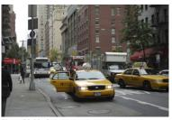
Figure 22.22. Curbside bus lanes often fail due to traffic congestion and poor enforcement (New York City). *ITDP*.
