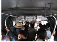
Figure 20.13. In cities, such as Quito and Bogotá, with relatively short average-trip distances, there can be more tolerance for having many standing customers. In cities with long travel distances, it can be quite tiring to customers. *Lloyd Wright*
