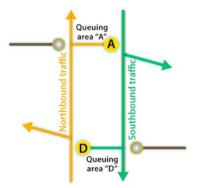
**Figure 24.63.** Vehicle movements for signal phase 2 in a cross converted into roundabout. *ITDP*.
