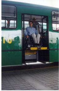
Figure 30.66. A special lift allows access for a wheelchair patron to a high-floor feeder vehicle in Bogotá. *TransMilenio SA*.
