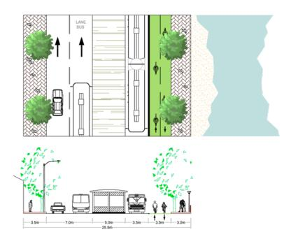
Figure 22.14. Plan and section view of Stretch 1 at a width of 25.5 meters. Logit.
