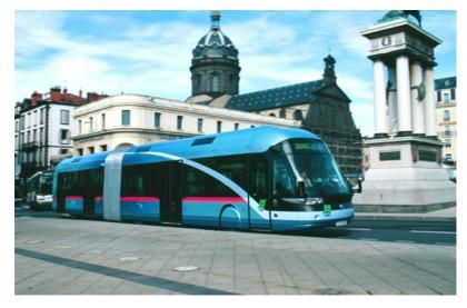
Figure 2.19. Modern vehicles can give BRT systems a highly professional image. The vehicle in this photo is a Civis bus in Clermont-Ferrand, France, and not a light-rail vehicle. US TCRP media library.
