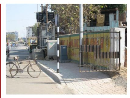
Figure 29.19. Sidewalk along a BRT corridor in Ahmedabad, India. While the gross width of the footpath is around two meters, obstructions reduce the usable clear width to zero meters. *ITDP*
