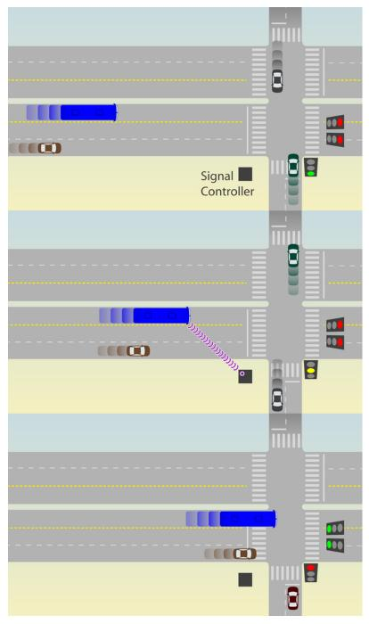
Figure 24.18. Active priority can reduce red time for the BRT corridor when the BRT vehicle is detected approaching the intersection. *ITDP*
