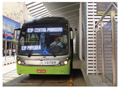
Figure 20.12. High-floor vehicles in conjunction with platform-level boarding have been the cost-effective solution for most high-quality systems in Latin America, such as the system in Belo Horizonte, Brazil. *ITDP*.
