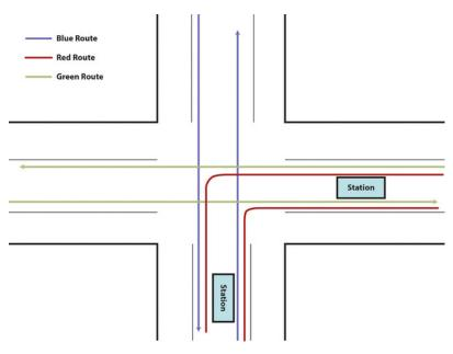
Figure 22.62. However, the required number of permutations becomes excessive, even for just a single intersection. Median stations permit easier platform transfers and multiple route permutations. *HHO Africa*.
