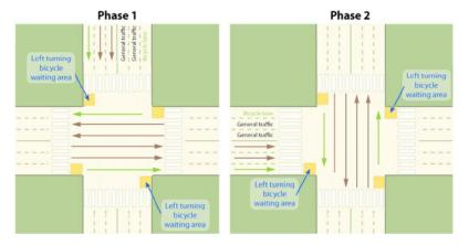
Figure 24.73. Schematic of the dedicated waiting area utilized for bicycles wishing to make cross-traffic turns in Xi'an. *ITDP*
