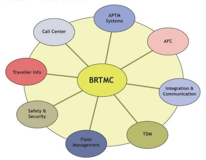
Figure 27.5. Typical functional elements of a BRTMC. Diagram ITDP.
