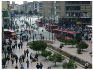
Figure 23.31. Textured and colored surface treatments help delineate pedestrian zones from roadways in Bogotá's BRT corridor. Karl Fjellstrom, Far East BRT
