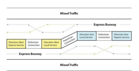
Figure 22.57. By offsetting the sub-stops and elongating the platform, passing lanes can fit into relatively narrow road widths. *Lloyd Wright*.
