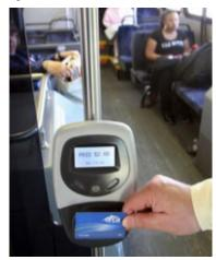
Figure 19.7. Onboard smartcard reader. ITDP
