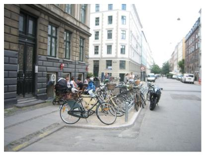
Figure 32.9. Bicycle-parking facilities can double as bollards and useful infrastructure for cyclists. Copenhagen, Denmark. *ITDP*.
