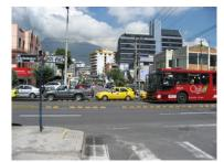
Figure 24.31. Prior to Quito's Ecovia line, mixedtraffic vehicles were allowed to cross through this intersection as well as negotiate cross-traffic and curbside turns. To give priority to public transport, crossing straight and cross-traffic turn movements have been blocked. *Lloyd Wright*.
