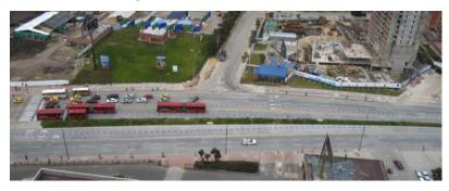
Figure 24.16. Single to double lanes just before the intersection in Bogotá to ensure proper capacity. Oscar Edmundo Diaz, GSD+.
