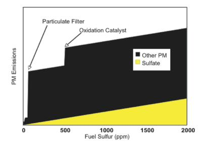
Figure 20.31. There is a close relationship between the emissions of sulfur and emissions of particulate matter (PM). Luis Willumsen.
