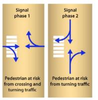
Figure 24.69. In a standard two-phase traffic signal, pedestrians are potentially at risk during both phases. *ITDP*.
