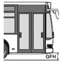
Figure 20.9. GFH 360 mm maximum; Low Entry; Short and Long Bus; *ITDP*
