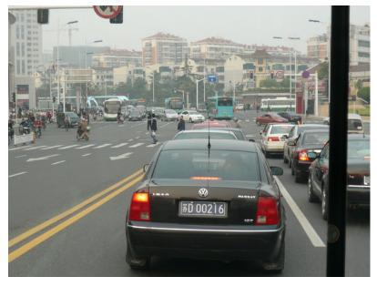
Figure 22.46. Changzhou, China, operates its BRT system along mixed-traffic lanes at a crucial segment of the corridor, and thus travel times and system control are negatively affected. *ITDP*.
