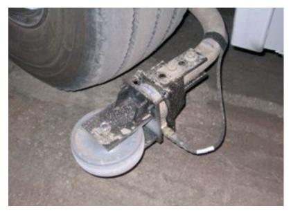
Figure 30.47. guide wheel in greater detail Cleveland RTA
