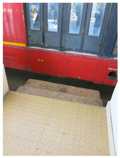
Figure 28.15. For customers transferring to and from the feeder busses that run in mixed traffic and are not high platform at Pimpri-Chinchwad's terminal, steps are built from the high platform of the station to the ground. *ITDP*
