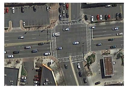
Figure 24.30. Lanes as narrow as 2.4 meters are an effective way to improve intersection capacity, as in this intersection in Montgomery County, Maryland, USA. *Google Earth*.
