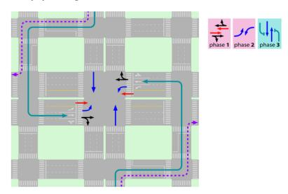
Figure 24.38. By detouring a cross-traffic turn to a curbside parallel street before reaching the intersection, a phase is eliminated in the main intersection. *Elebeta*.
