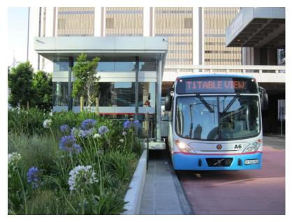
Figure 25.94. Cape Town uses Kassel curbs, a sloped curb that minimizes the wear and tear on the tires of the bus by curving up. *ITDP*
