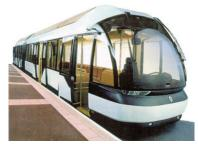
Figure 20.41. Despite giving a distinctly light-rail appearance, the Civis vehicle is actually a bus. US TCRP media library.
