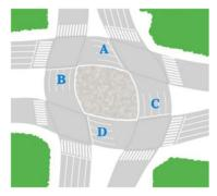
Figure 24.61. In this scenario, the intersection is converted to a roundabout with vehicle queuing areas at points "^, "B," "C," and "D." The BRT vehicles enter mixed traffic just before the intersection and move through the intersection with a two-phase signal. *ITDP*
