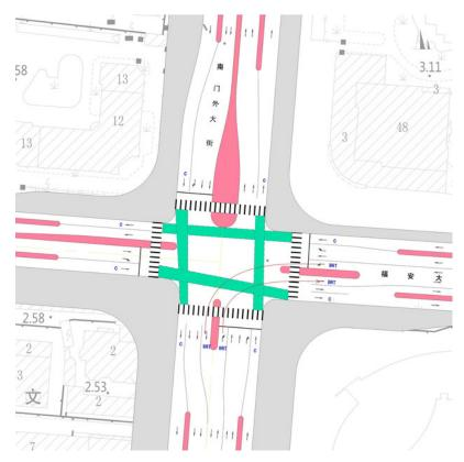
Figure 31.23. A design for cycle lanes and BRT at an intersection in Tianjin, China. Note the green bike lanes extend through the intersection, and that the side medians end, allowing for a center median. *ITDP*.
