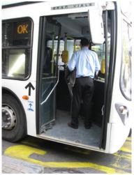
Figure 20.10. Low-floor vehicles without platformlevel entry and pre-board fare verification can result in longer dwell times and not actually provide access to the physically disabled, as shown in this image from Santiago, Chile *Lloyd Wright*
