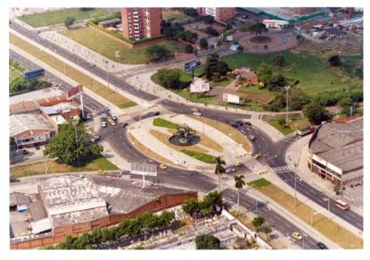
Figure 24.68. In Cali, the busway also passes through the center of the roundabout area. Metrocali.
