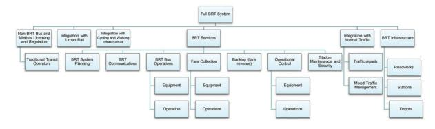
Figure 12.1. Basic functions of a full BRT system. Walter Hook, BRT Planning International, LLC.
