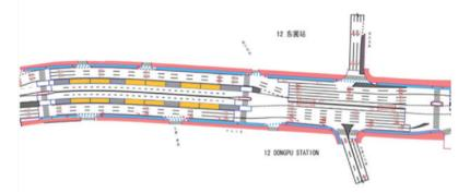
Figure 24.45. Dongpu BRT station in Guangzhou, provides at-grade station access at both ends, combined with U-turns. *ITDP with GMEDRI*.
