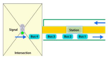
Figure 24.26. For the direction of the BRT system that stops after the intersection, there is a risk that vehicles create a backup into the intersection and block traffic. *ITDP*.
