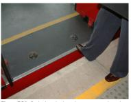
Figure 7.21. Reducing the borad gap, as seen here in Bogotá, Colombia, allows customers to safely board and alight faster, increasing system capacity. *Lloyd Wright*.
