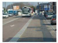
Figure 22.43. The virtual lane concept in Rouen, France, where a single centrally located bus lane is used to provide bus priority in both directions of travel. Andre Frieslaar.
