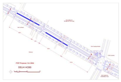
Figure 24.22. In this proposed road layout for Delhi, the mid-block BRT stations are given additional right-of-way and several access points. At the intersections, right-of-way for vehicles in mixed traffic is maximized. *ITDP*.
