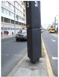
Figure 29.48. This BRT-identification post in Quito is placed in a pedestrian island, and acts to block the pedestrian's view of both oncoming mixed traffic as well as oncoming BRT vehicles. *Lloyd Wright*
