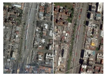
Figure 25.35. The image on the left is the Calle 100 station in 2005 with just two sub-stops, but space for more. The image on the right is the same station in 2013 with an additional sub-stopn having been added due to increased demand. *Google Earth.*
