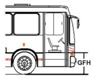
Figure 20.7. GFH 960 mm maximum Long Bus; Rear Engine High Floor *ITDP*
