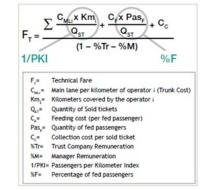
Figure 15.10. Detailed form of technical fare calculation; passengers per kilometer index. *TransMilenio*
