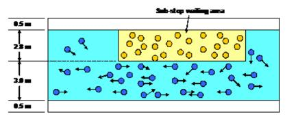
Figure 25.54. Platform width example *ITDP*
