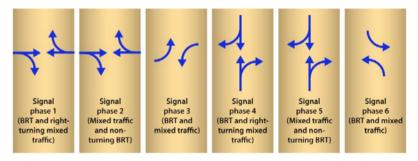
Figure 24.56. To permit a full range of both BRT and mixed-traffic turning movements, six signal phases would be required. *ITDP*.
